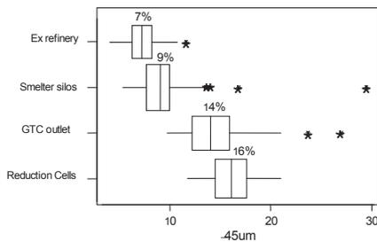
Figure 5 – Particle Breakdown and Fines Variation Within a Smelter
