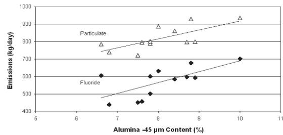
Figure 6 – Impact of Fines in Primary Alumina on Particulate and Fluoride Emissions
