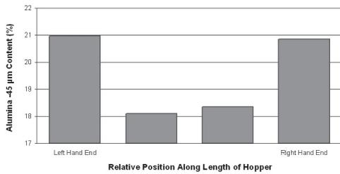
Figure 4 – Fines Segregation in the Reduction Cell Hoppers
