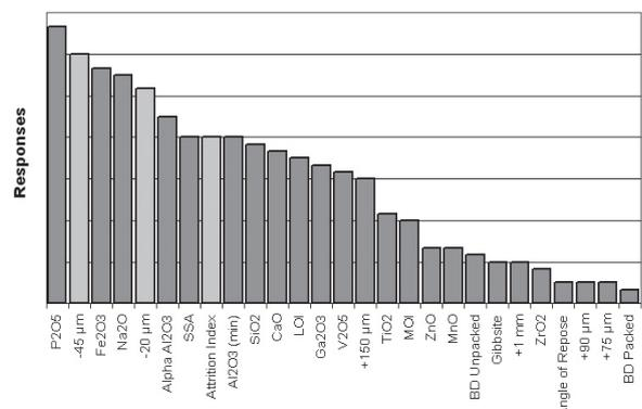
Figure 1 – Alumina Characteristics in Order of Importance from Smelter Perspective
