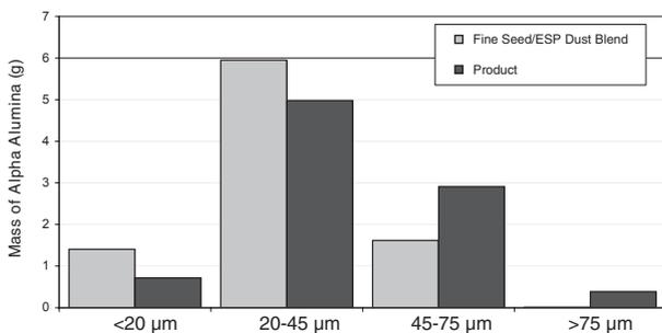
Figure 2 – Growth of ESP Dust in Precipitation as Traced by Alpha Alumina Content
