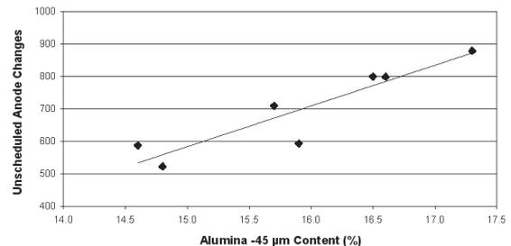
Figure 7 – Impact of Fines in Secondary Alumina on Unscheduled Anode Changes
