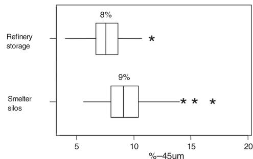
Figure 3 – Fines Content in Storage Silos at Refinery and Smelter
