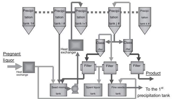
Figure 2 Schematic flow sheet of the pregnant liquor diffidence process
