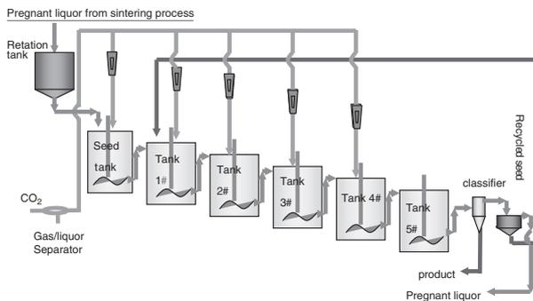
Figure 4 Schematic flow sheet of Continuous Carbonation Precipitation Technology
