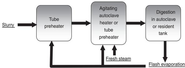
Figure 1 Schematic flow sheet of Tube-Preheater with Autoclaves or Retention Tanks
