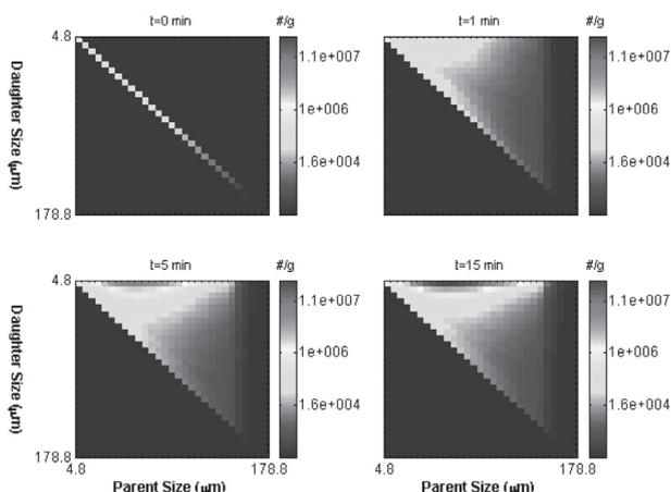
Figure 10. Breakage maps at different attrition times for Sample D, linking the parent size and daughter particle size.
