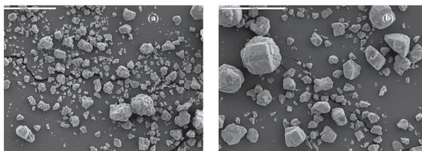
Figure 9. SEM images of the breakage products after 15 minutes in the Hertwig-Forsythe unit for (a) Sample D and (b) Sample A.
