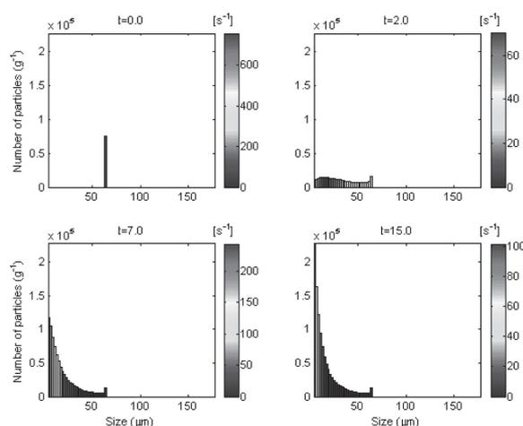
Figure 12. Breakage activity plots at different attrition times for a narrow size interval at 60 µm from Sample A.
