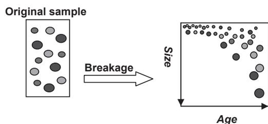
Figure 4. Conceptual model of breakage process; colour depicts the size of original parent particle.
