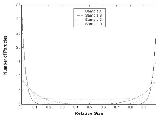
Figure 8. Estimated number-based breakage distribution functions for the four alumina samples.
