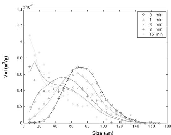
The results in Figure 5 show typical level of the agreement observed with the samples analysed to date. These two tests, i.e. to match the breakage PSD and the distribution of the tracer at various attrition times, are particularly challenging. Very good agreement between the model and experimental data has been observed for the 15 alumina samples analysed to date.
