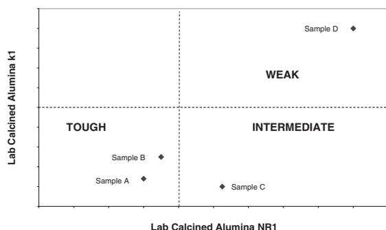
Figure 1. ‘Toughness plot’ comparing the relative attrition resistances of the four aluminas being investigated.
