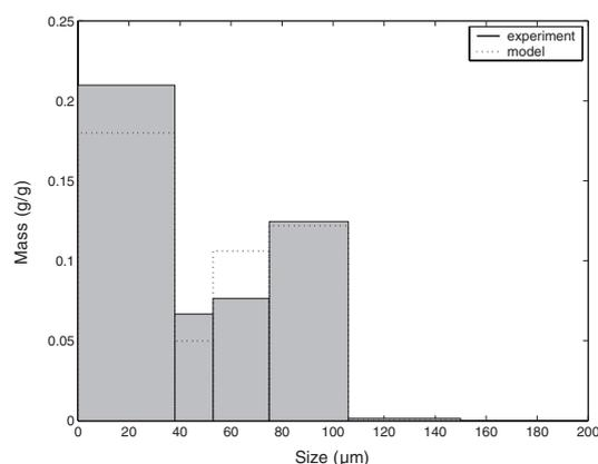
Figure 5. (a) Experimental (symbols) and model predicted (lines) PSD at different attrition times. (b) Experimental and model predicted Cu tracer size distribution after 15 minutes of attrition (Sample D)
