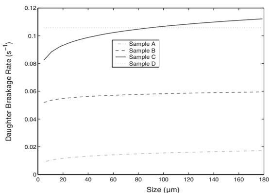
Figure 7. Comparison of the daughter particle breakage rates for the four alumina samples.
