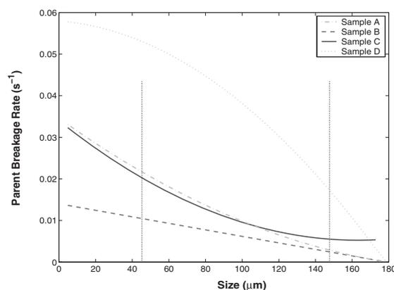
Figure 6. Comparison of the parent particle breakage rates for the four alumina samples. Most of the mass in the samples is distributed between 50 µm and 150 µm, as marked by the vertical dashed lines.
