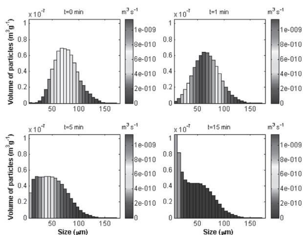
Figure 11. Breakage activity plots at different attrition times for Sample D, showing the changing PSD and the breakage rate intensities within the different size intervals.
