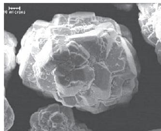
Figure 1: SEM image of the as received gibbsite seed
