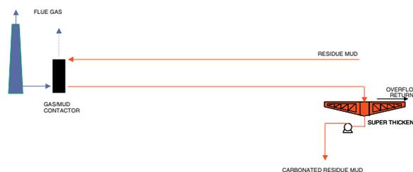
Figure 3: Mix flue gas into a dilute slurry
