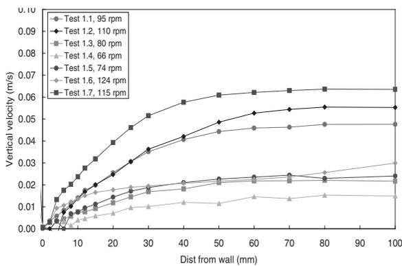
Figure 6. Vertical component modified and original configurations 960 mm above base of tank. Same power as benchmark case.
