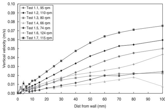
Figure 5. Vertical component modified and original configurations 297 mm above base. Same power as benchmark case.
