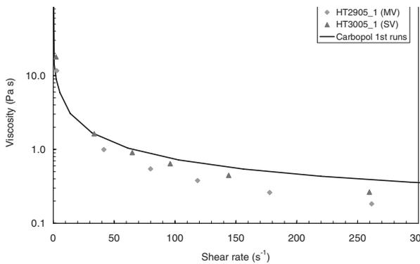
Figure 2. Comparison between Carbopol used for initial tests and rheology of typical bauxite slurry. Viscosity vs shear rate.
