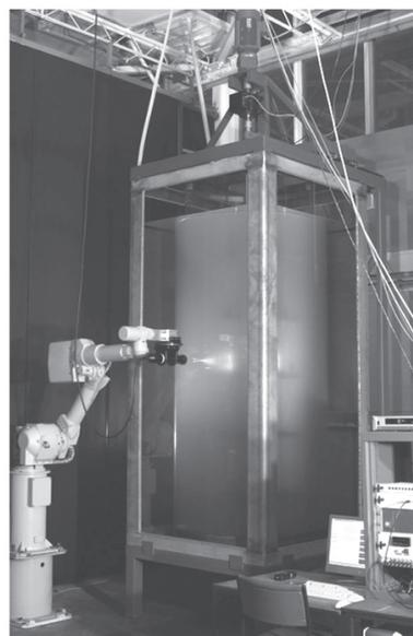
Figure 1. View of 1.0 m diameter 3.0 m tall tank (high aspect ratio) and robot mounted LDV system.
