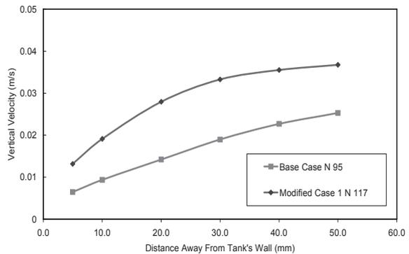
Figure 8. Velocity profiles for original and modified cases. 400 mm from bottom for liquid level 2350 mm.
