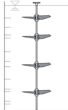
Figure 4. Benchmark case impellers with dashed lines showing where LDV measurements made.
