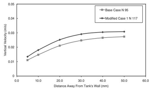
Figure 9. Velocity profiles for original and modified cases. 900 mm from bottom for liquid level 2350 mm.
