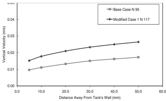
Figure 10. Velocity profiles for original and modified cases. 2000 mm from bottom for liquid level 2350 mm.
