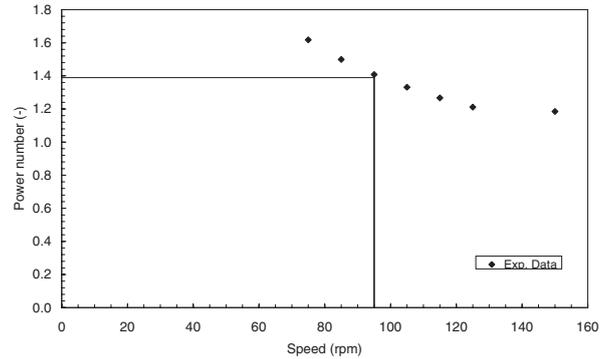
Figure 3. Power number versus speed for Carbopol in 1.07 m tank. 95 rpm selected as operating speed in the physical model to give the same power number as a full size tank.
