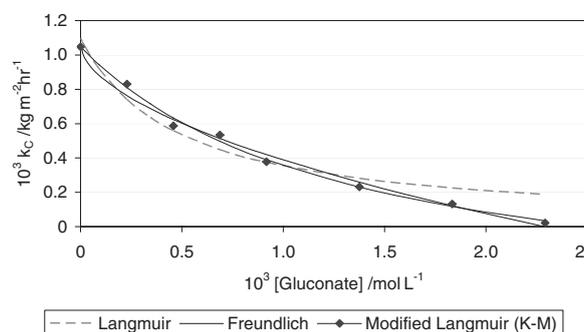
Figure 2. Crystal growth rate as a function of sodium gluconate concentration. Initial TC 195–205 gL<sup>-1</sup> (as Na<sub>2</sub>CO<sub>3</sub>), gibbsite seed 100 gL<sup>-1</sup>, 70°C and  $g = 2.8$ .
