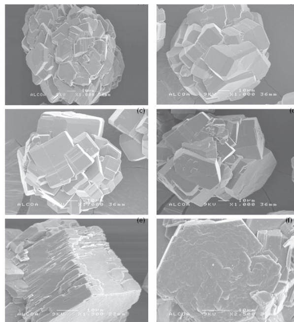
Figure 3. Electron micrographs of gibbsite crystals grown in the presence of sodium gluconate: [left to right] (a) seed crystal; (b) crystal after 50 hours in the absence of gluconate; (c) crystal after 50 hours with  $50 \text{ mg L}^{-1}$  sodium gluconate; (d) crystal after 50 hours with  $200 \text{ mg L}^{-1}$  sodium gluconate; (e), (f) crystals after 50 hours with  $500 \text{ mg L}^{-1}$  sodium gluconate.
