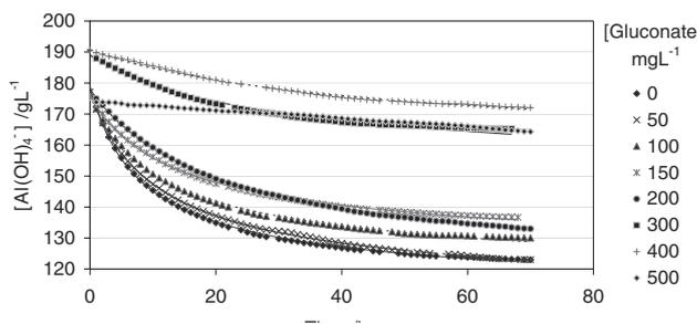
Figure 1. Aluminate de-supersaturation data as a function of time in the presence of varying concentrations of sodium gluconate. Initial TC 195–205 gL<sup>-1</sup> (as Na<sub>2</sub>CO<sub>3</sub>), gibbsite seed 100 gL<sup>-1</sup>, 70°C. Fitted curves shown for  $g = 2.8$ .
