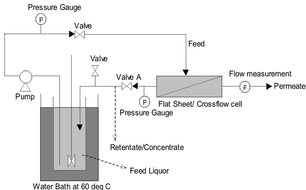
Figure 1 — Flowsheet of the flat sheet membrane test rig.
