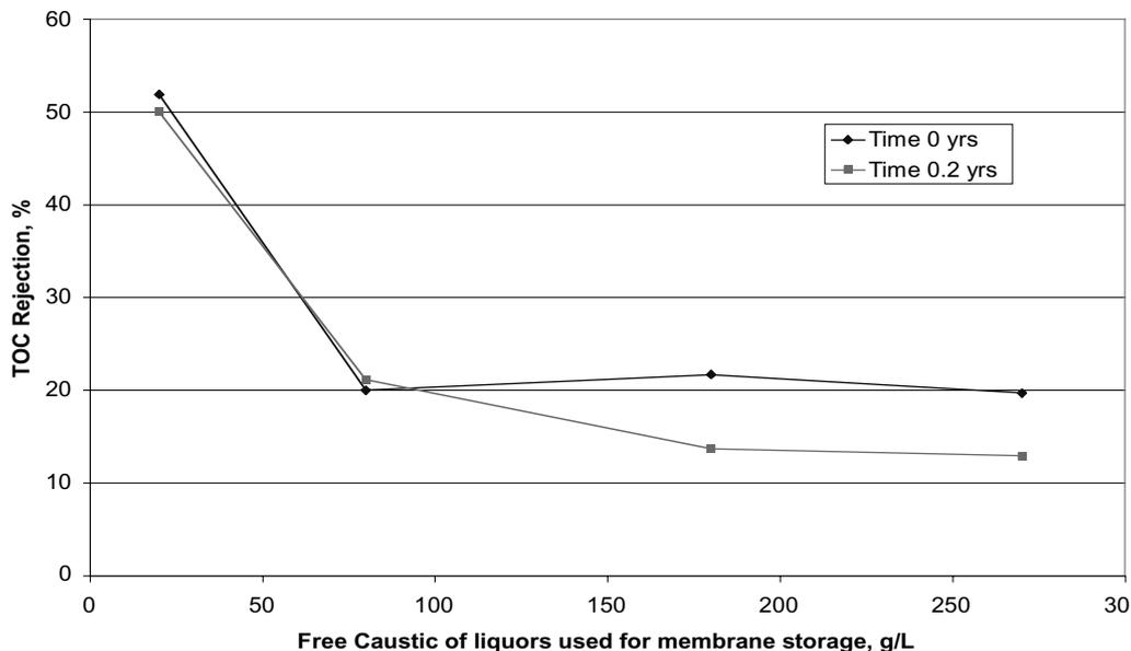
Figure 7 — TOC rejection versus free caustic at zero and 0.2 years storage (for P005F).
