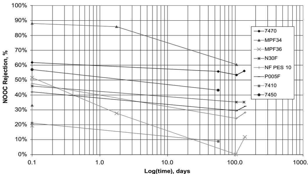
Figure 3: — NOOC rejections from seed wash filtrate feed (B filtrate).
