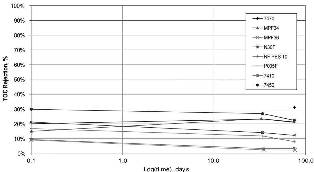
Figure 4 — TOC rejections from a diluted L-D feed after storage in 80g/L free caustic.
