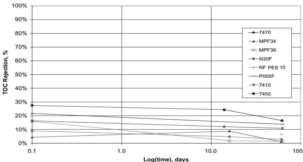
Figure 5 — Repeat TOC rejections from an L-D feed after storage in ~180g/L free caustic solution.
