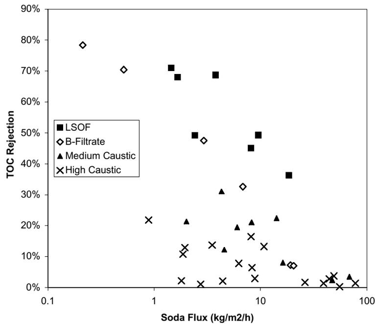
Figure 6 — Membrane TOC rejection as a function of soda flux.
