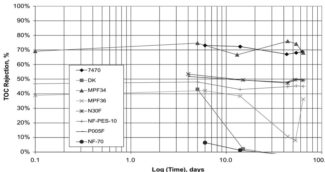
Figure 2: — TOC rejections from a lime treated seed wash feed (LSOF).
