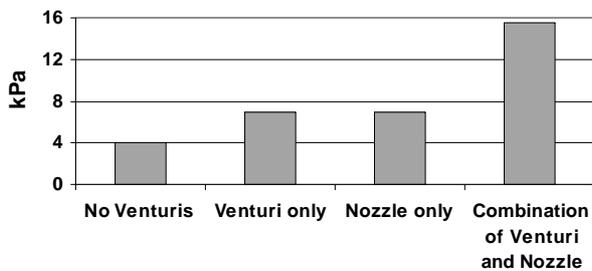
Figure 5 — Impact of venturis and straightener nozzles on peak cleaning pressure from laboratory tests.
