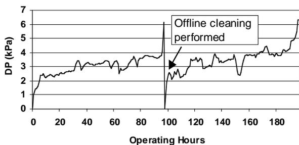
Figure 2 — Baghouse Differential Pressure drift.
