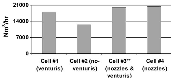
Figure 6 — Gas flows achieved through each cell with different cleaning system in each cell of the baghouse (\*\* 350 kPa air supply pressure with other cells at 650kPa).
