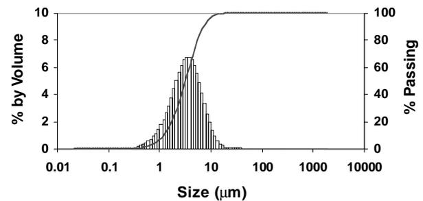
Figure 3 — Typical Dust Size Analysis of Baghouse Feed.
