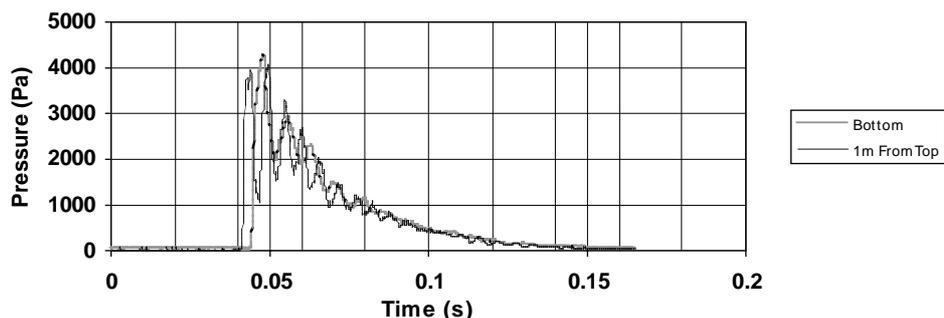
Figure 4 — Cleaning pressure profile achieved on element.
