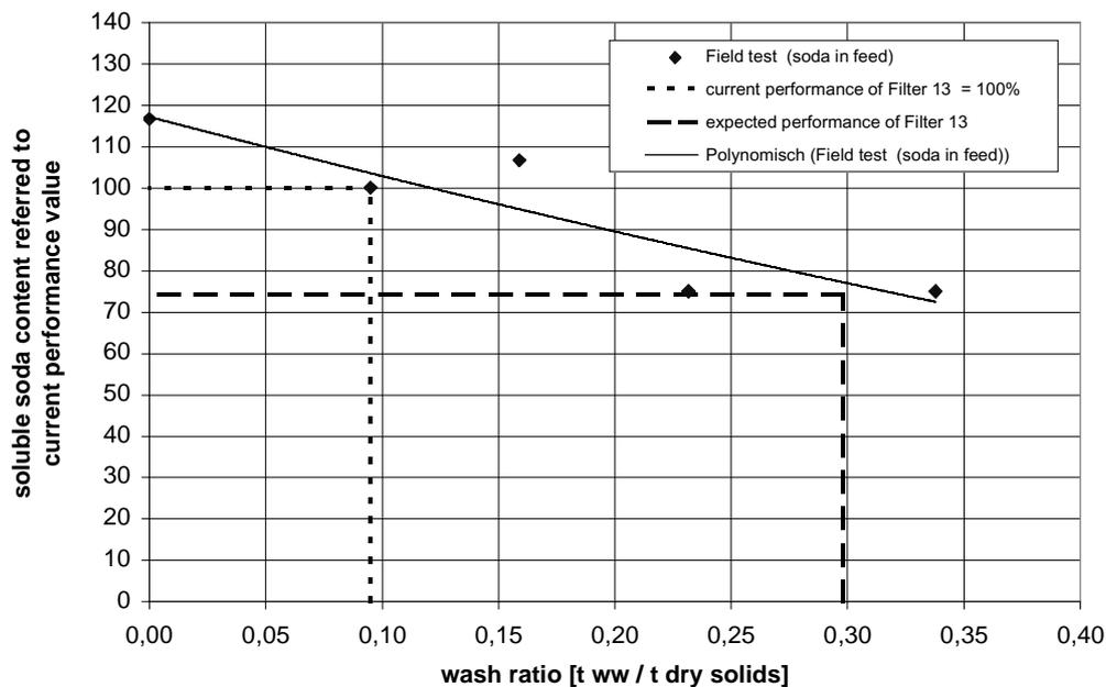
Figure 5 — Operation value and expected value of soluble soda content in the cake versus wash ratio
