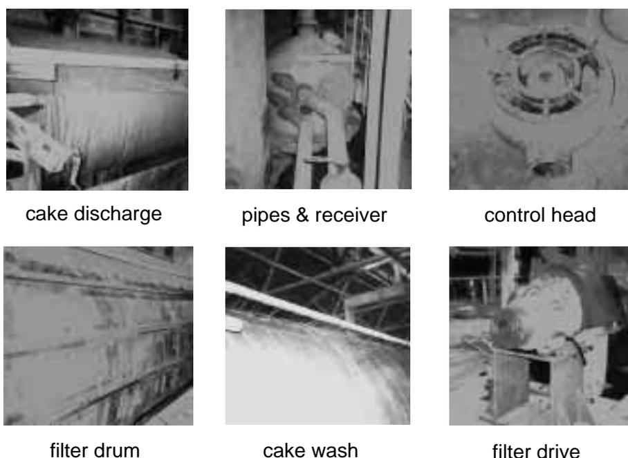
Figure 6 — View of some parts to modify for revamping of the red mud drum filter
