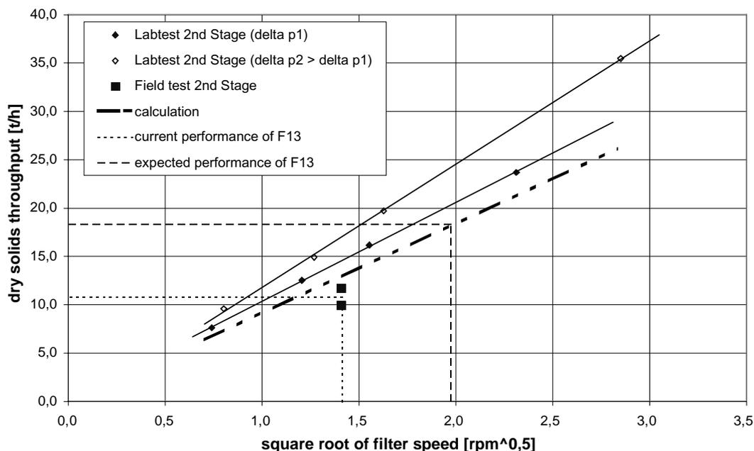
Figure 4 — Operation value and expected value for solids throughput versus square root of filter speed
