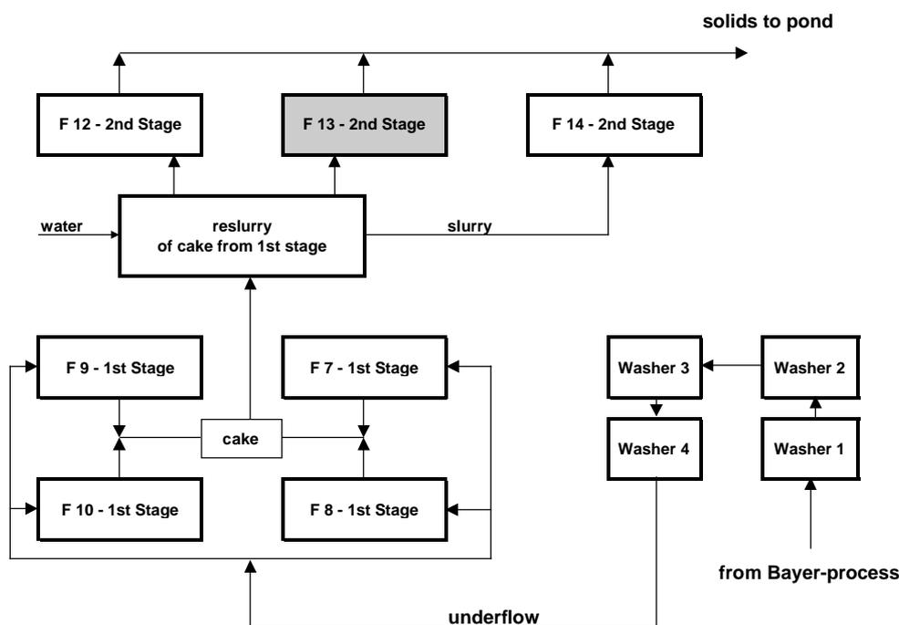
Figure 3 — Flow sheet of the red mud filtration Line 1 (solids to pond)
