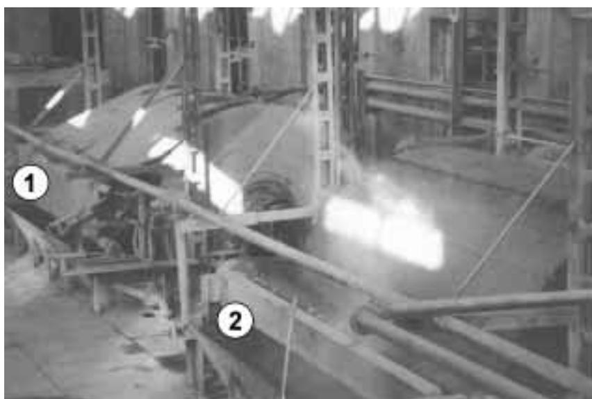
Figure 7 — Drum filter before the upgrading with belt discharge (1) and drum filter upgraded by BOKELA with roller discharge (2)
