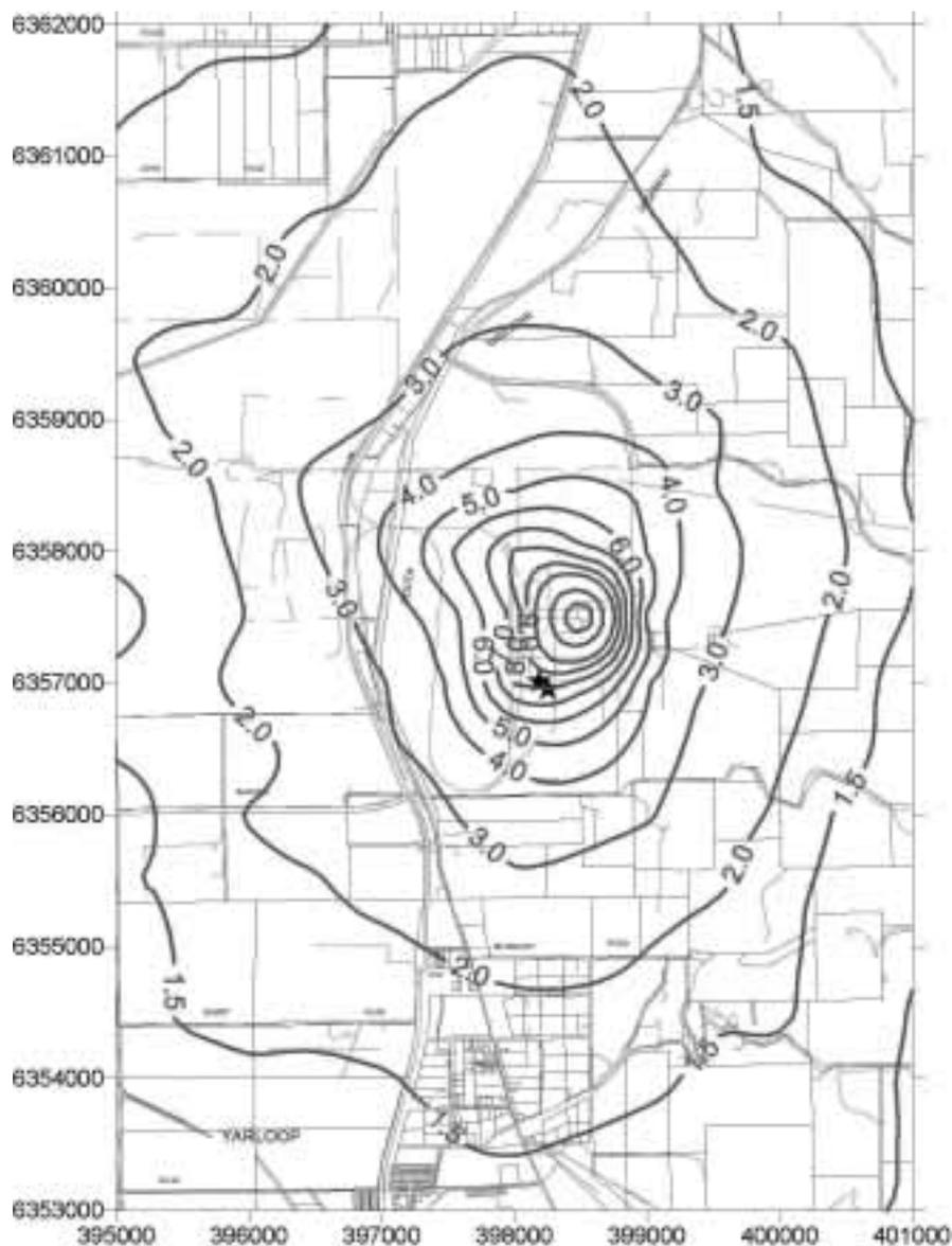
Figure 4 — Predicted 3-minute 99.5 percentile ground level concentration from Wagerup Refinery using the 2000 odour survey
