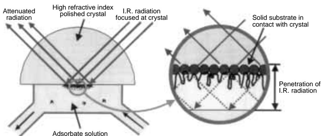
Figure 1 — Schematic representation of the ATR cell, showing the deposited hematite colloid and flocculant adsorbed from the synthetic liquor (applied at a constant flowrate).
