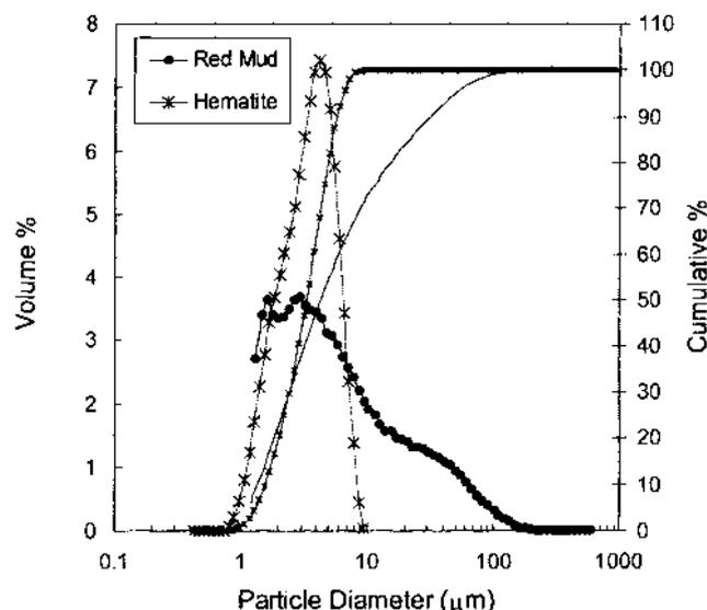
Figure 4 — Particle size distribution of unflocculated hematite and red mud suspensions
