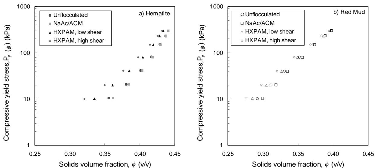
Figure 3 — Compressive yield stress results for hematite and red mud suspensions
