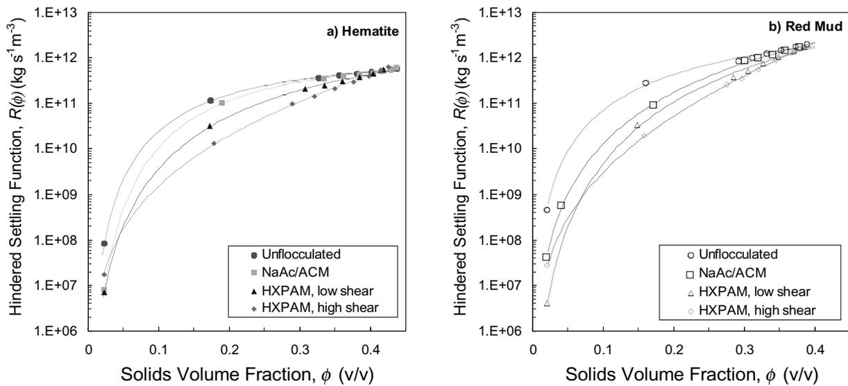
Figure 5 — Hindered settling function curves for hematite and red mud suspensions
