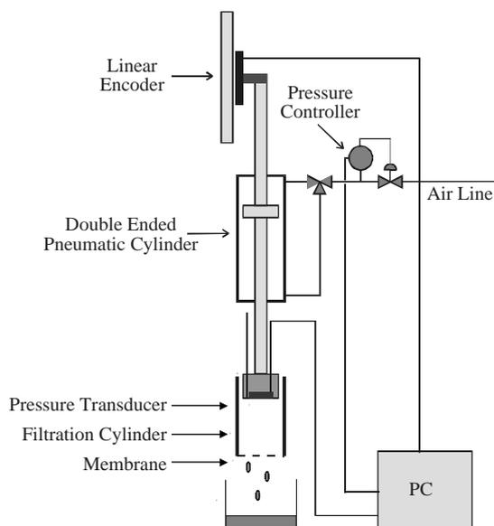
Figure 1 — Schematic of the automated stepped pressure filtration rig used for permeability and compressibility measurements
