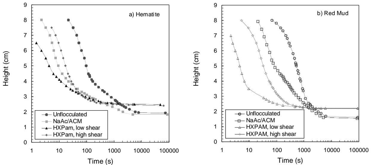
Figure 2 — Interface height versus time results for hematite and red mud suspensions
