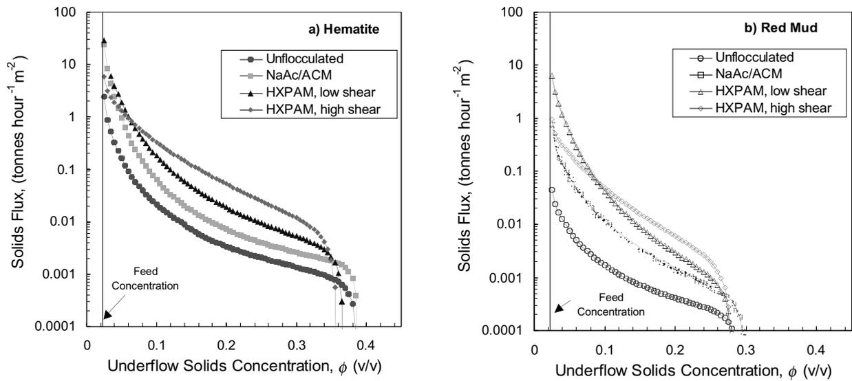
Figure 6 — Solids flux versus underflow solids concentration for hematite and red mud suspensions
