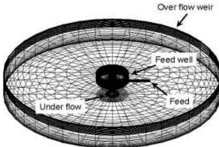
Figure 1 — Grid for the CFD model of the 1<sup>st</sup> washer at Aughinish
