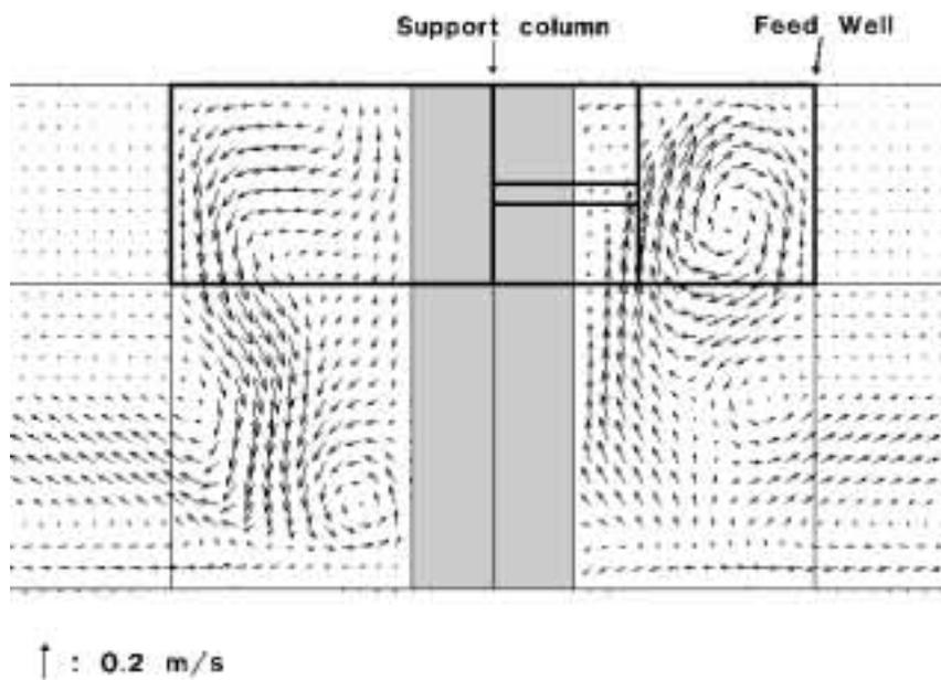
Figure 3 — Liquid vector field in the feed well area, for the simulation of the feed pipe integrated with the wall of the feed well, for the 1<sup>st</sup> washer at Aughinish
