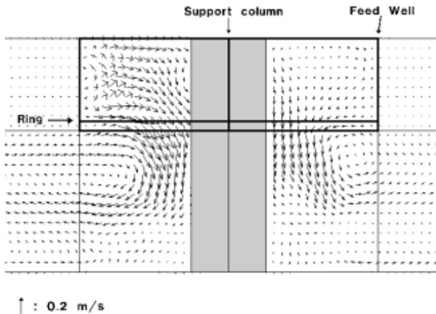
Figure 5 — Liquid vector field in the feed well area, for the simulation of the effect of an annular ring and overflow recirculation, for the 1<sup>st</sup> washer at Aughinish
