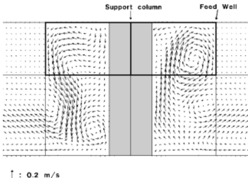
Figure 2 — Liquid vector field in the feed well area, for the simulation of the base case, for the 1<sup>st</sup> washer at Aughinish
