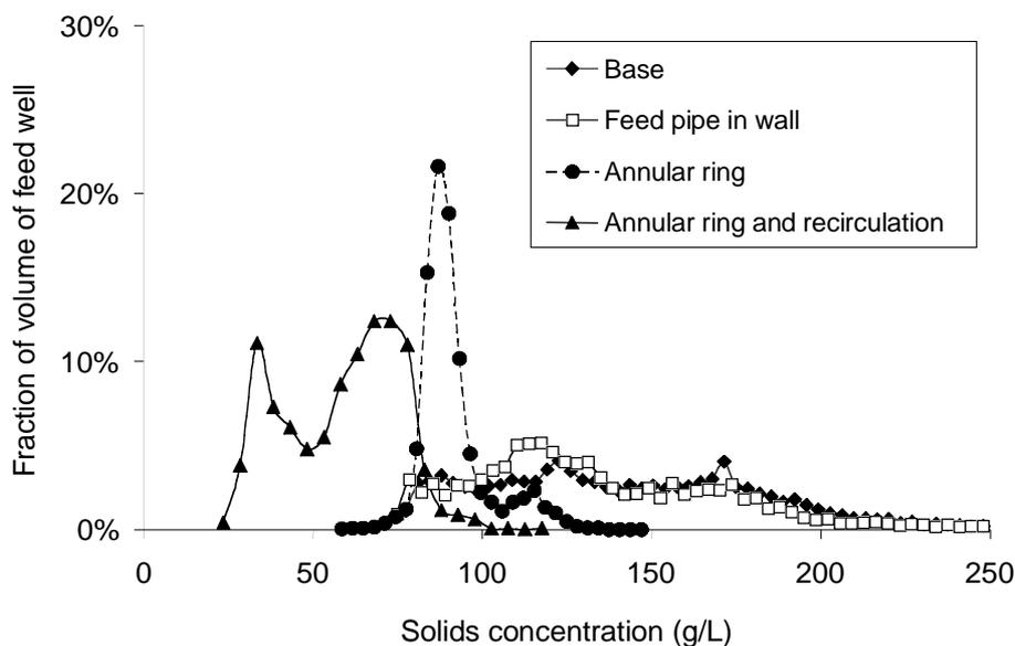
Figure 6 — Distribution of solid concentration in the feed well for the cases simulated, for the 1<sup>st</sup> washer at Aughinish
