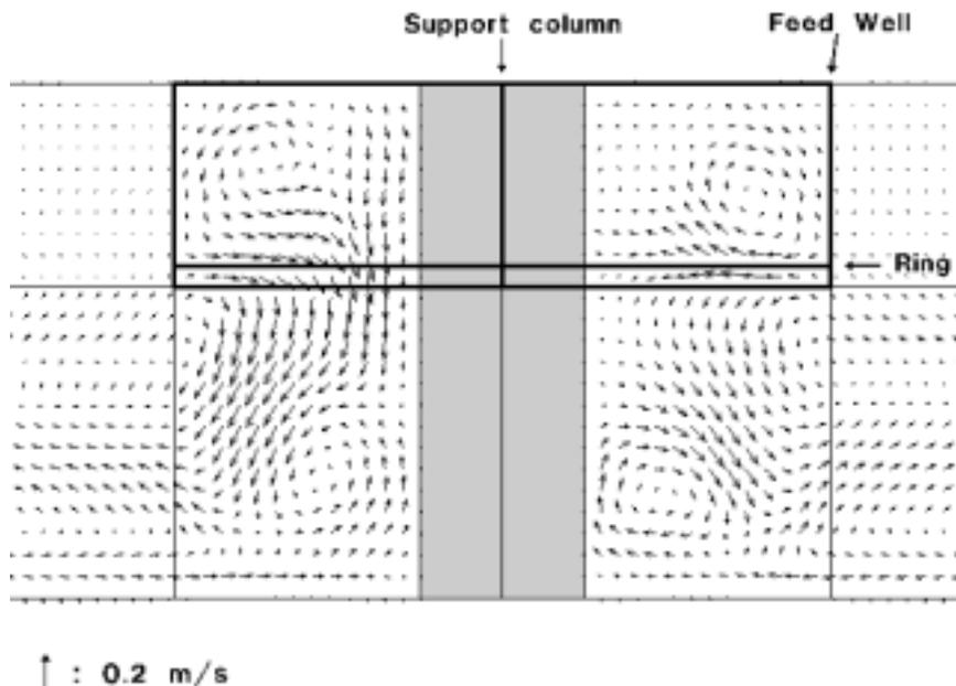
Figure 4 — Liquid vector field in the feed well area, for the simulation of the effect of an annular ring, for the 1<sup>st</sup> washer at Aughinish
