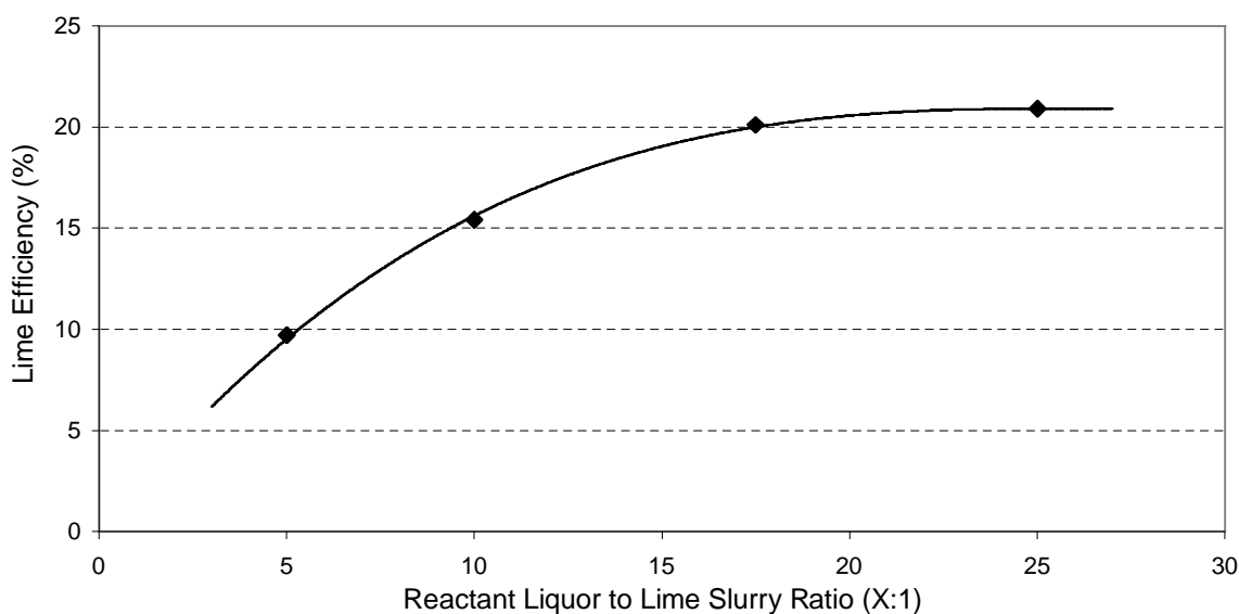
Figure 6 — Effect of varying the ratio of reactant liquor volume to lime added on fluoride removal
