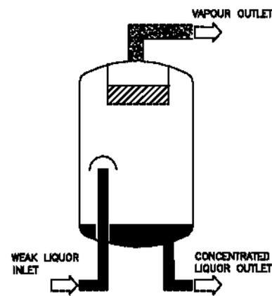
Figure 4 — Flash Evaporator
