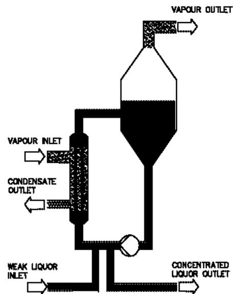
Figure 3 — Forced Circulation Evaporator
