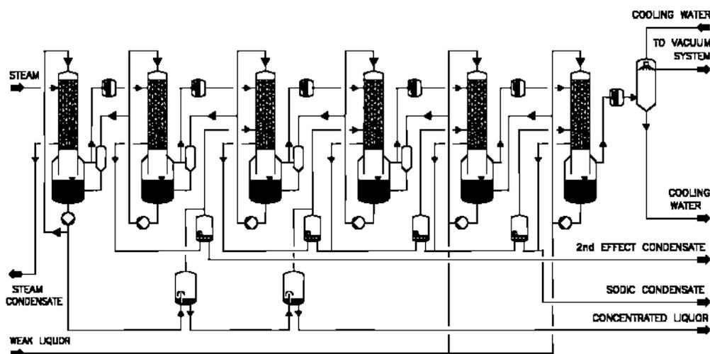
Figure 5 — Six Effect Falling Film Evaporation Plant
