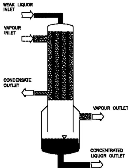
Figure 2 — Falling Film Evaporator
