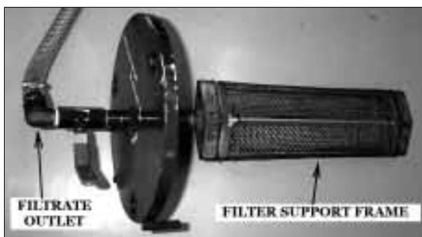
Figure 3 — Pilot Filter — filter frame
