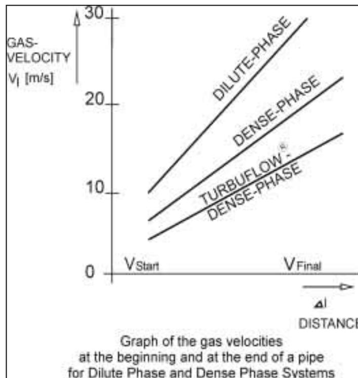
Figure 2 — Conveying velocities of different pneumatic transport systems
