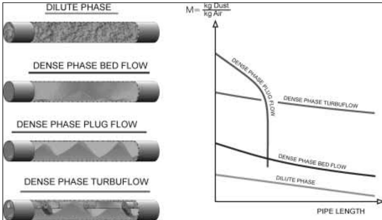
Figure 4 — Material/air rates for different pneumatic conveying systems
