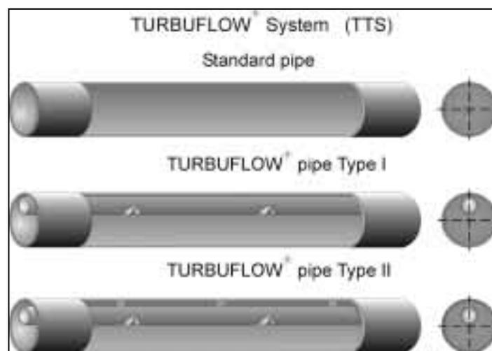
Figure 3 — The TURBUFLOW® Dense Phase feeding system
