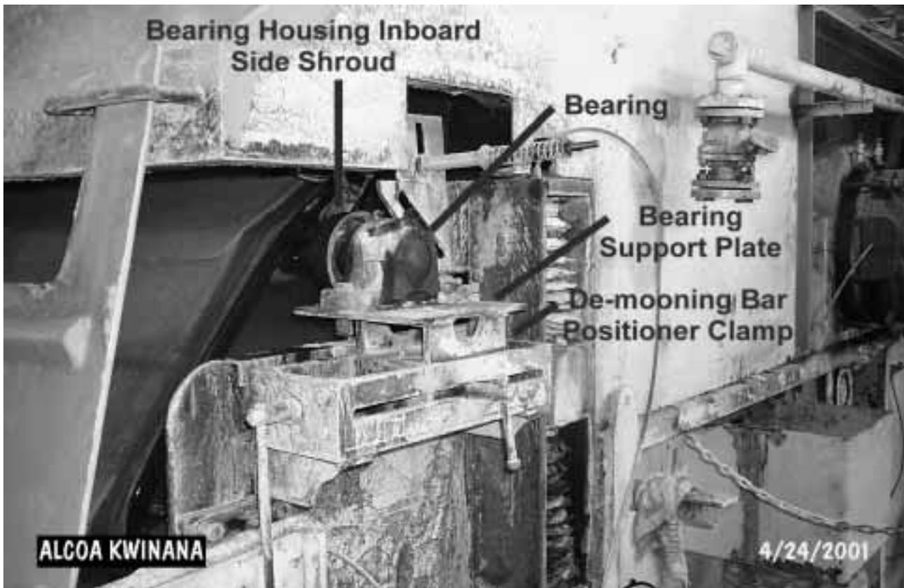
Figure 3 — New Discharge Roller System
