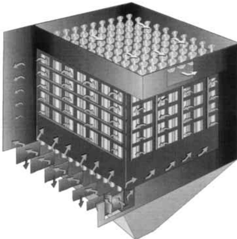
Figure 2 — Gas and Dust distribution in FabriClean Filters, figure is illustrating one half compartment. Arrows show direction of gas.
