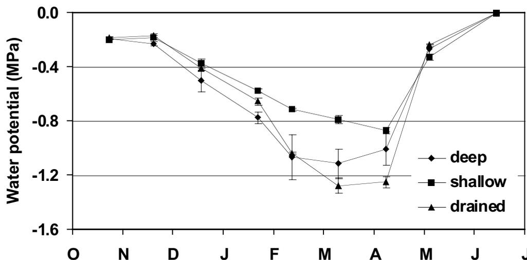
Figure 3 — Predawn leaf water potentials of trees on each of the deep, shallow, and drained lysimeters measured using a pressure chamber over the study period from October 2001 to May 2002.
