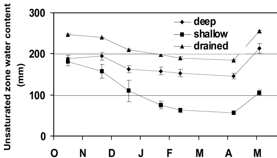
Figure 2 — Total water content in the unsaturated zone measured by neutron water meter in the shallow, deep and drained lysimeters over the study period from October 2001 to May 2002.
