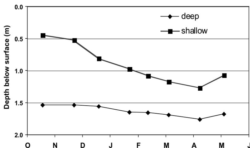
Figure 1 — Depth to the watertable measured in the shallow and deep lysimeters over the study period from October 2001 to May 2002
