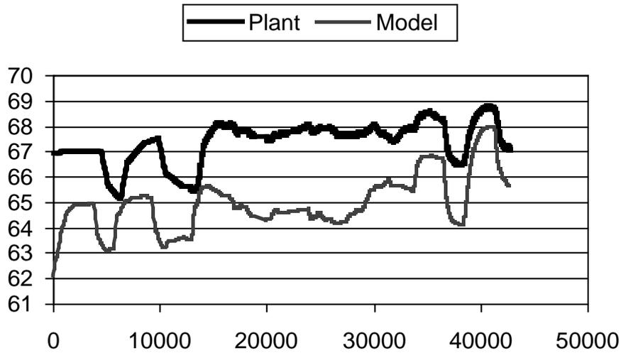
Figure 6 — 2nd Barometric flash vessel temperature trends; Model vs Plant.
