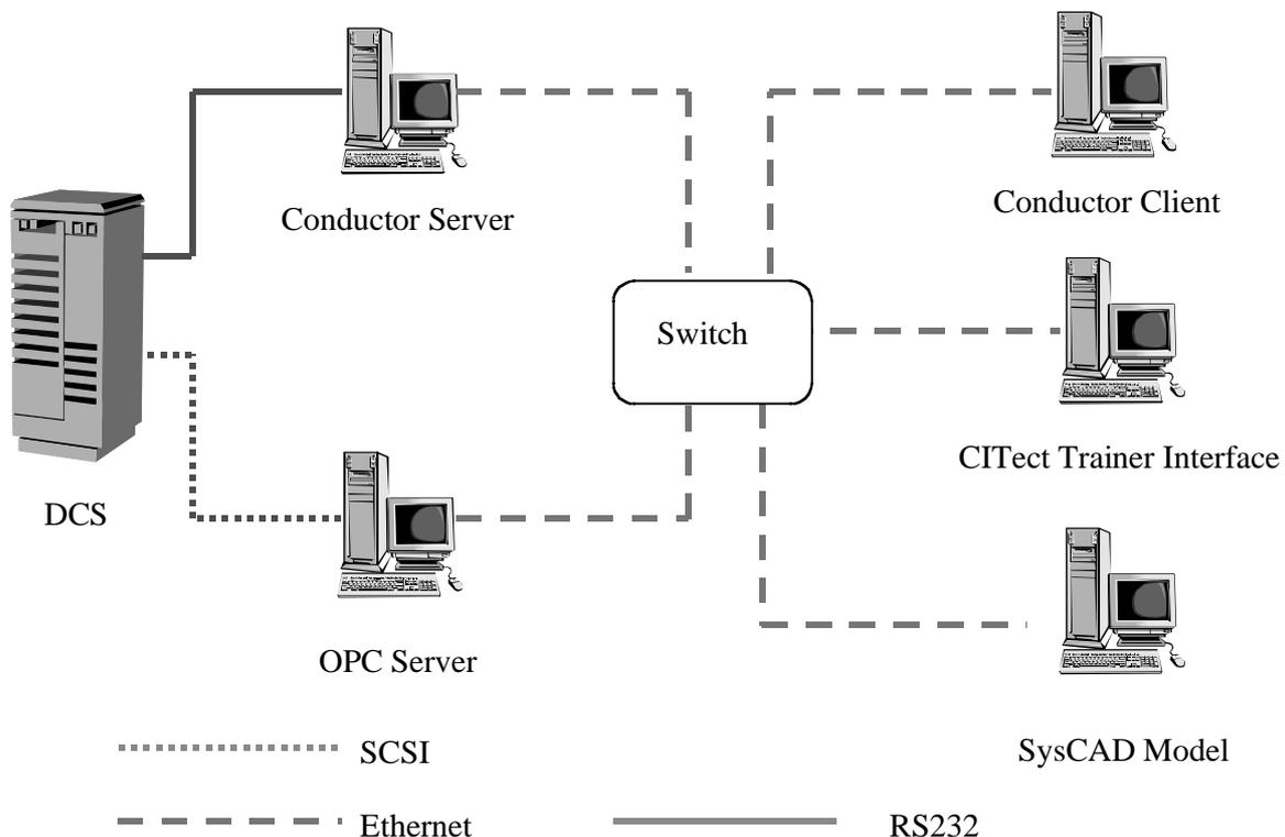
Figure 7 — Schematic of Evaporation Simulation system.
