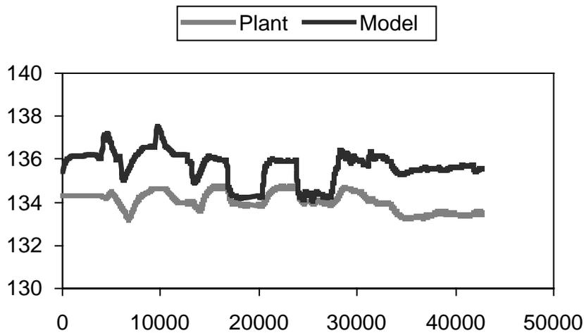
Figure 4 — 1<sup>st</sup> Flash vessel temperature trend; Model vs Plant.
