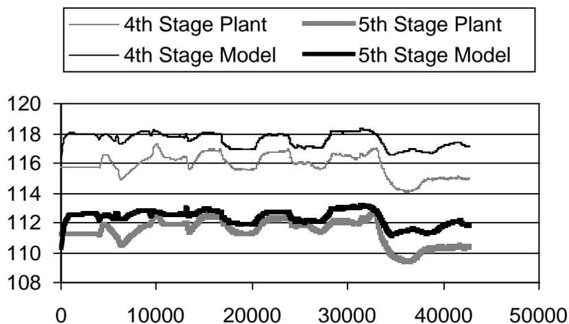
Figure 5 — 4<sup>th</sup> and 5<sup>th</sup> Flash vessel temperature trends; Model vs Plant.
