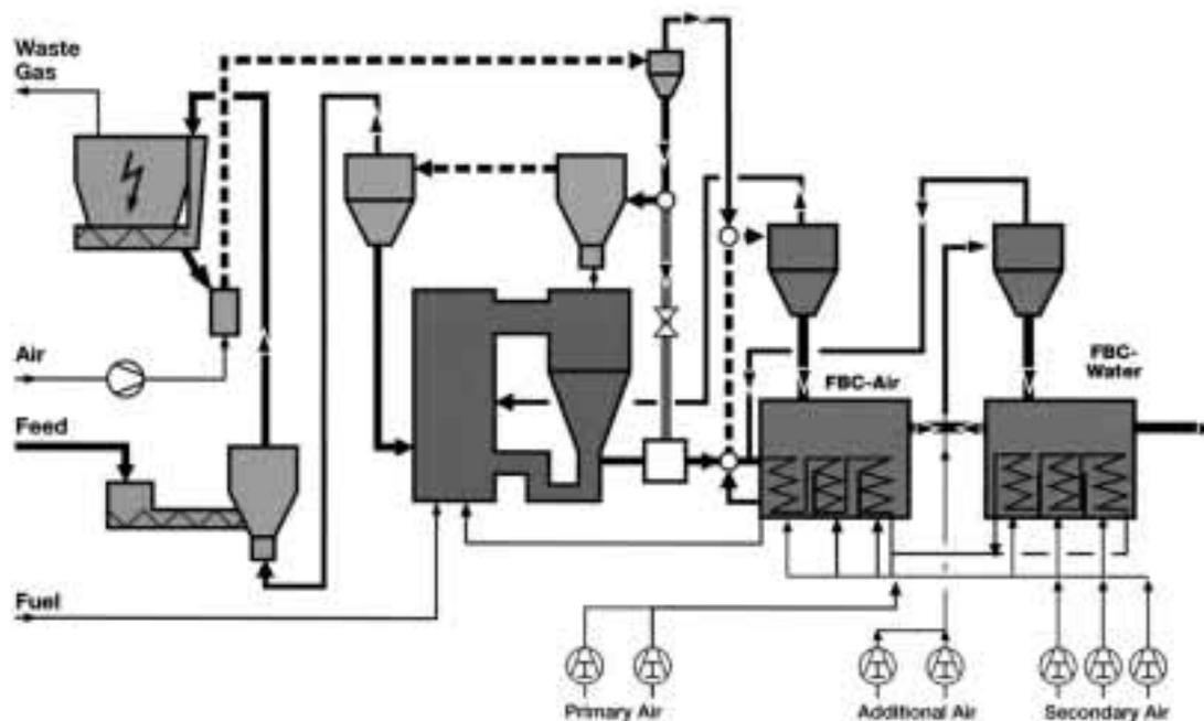
Figure 2 — Schematic of the Fluid Bed Calciner.
