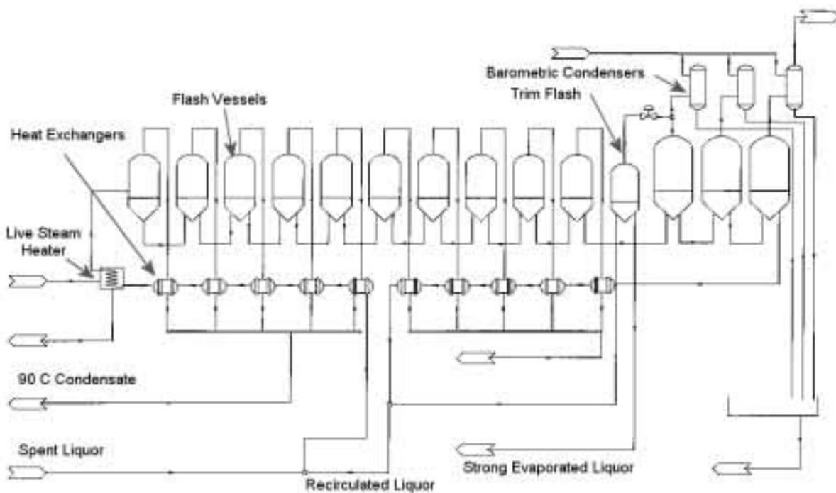
Figure 3 — Schematic of the Evaporation plant.
