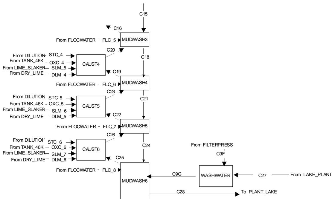
Figure 3 — Level of flowsheeting detail — example from model mud washing section
