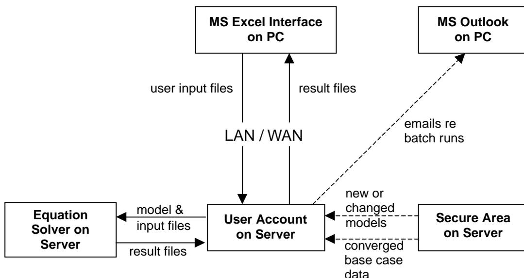
Figure 2 — Information Flows in a System for Widespread Access to a Centrally Managed System of Models
