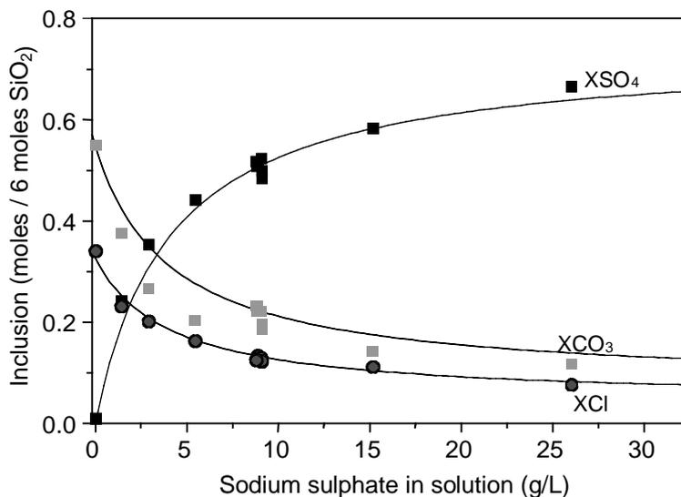
Figure 4 — Inclusion of equations to describe process chemistry: DSP composition example
