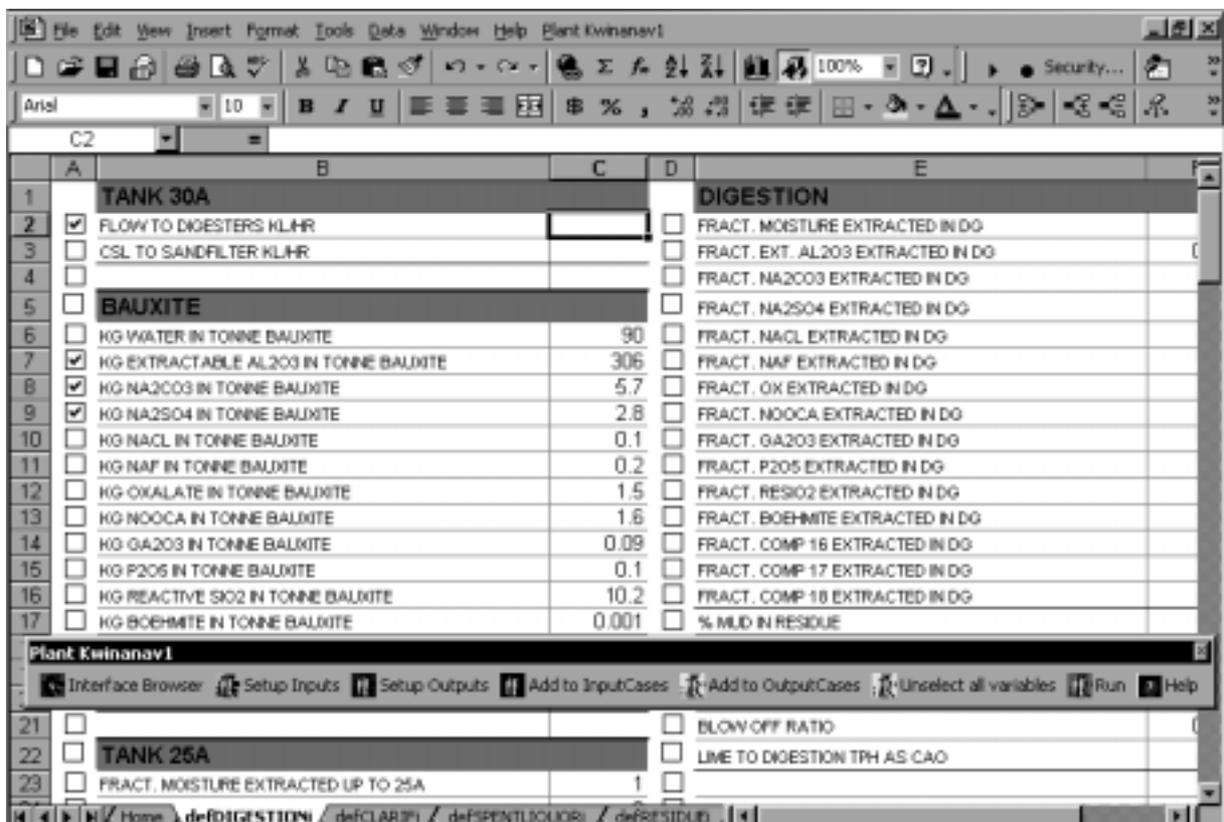
Figure 1 — A Snapshot from the Excel User Interface for a Plant Impurity Balance Model
