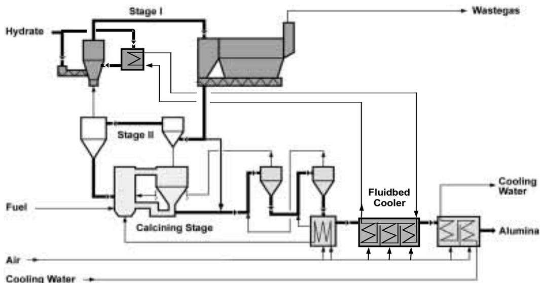
Figure 6 — Heat Transfer from FBC to Hydrate Dryer
