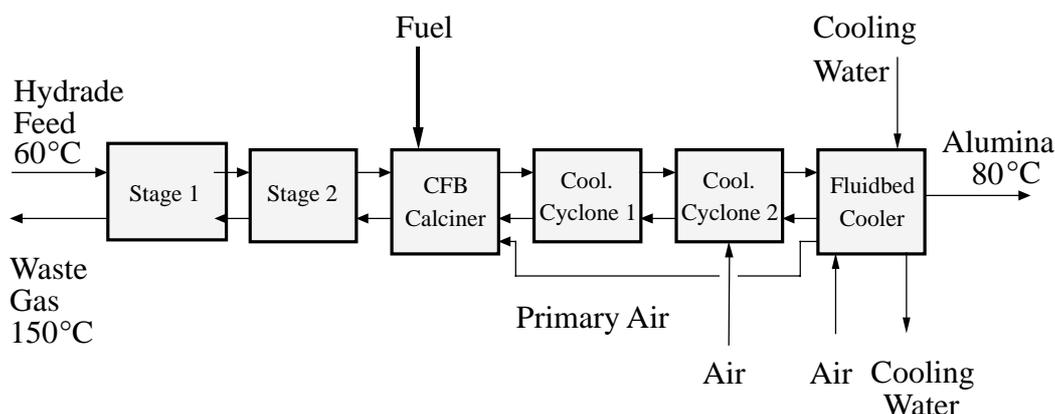
Figure 4 — Block Diagram of the CFB — Calcination Process
