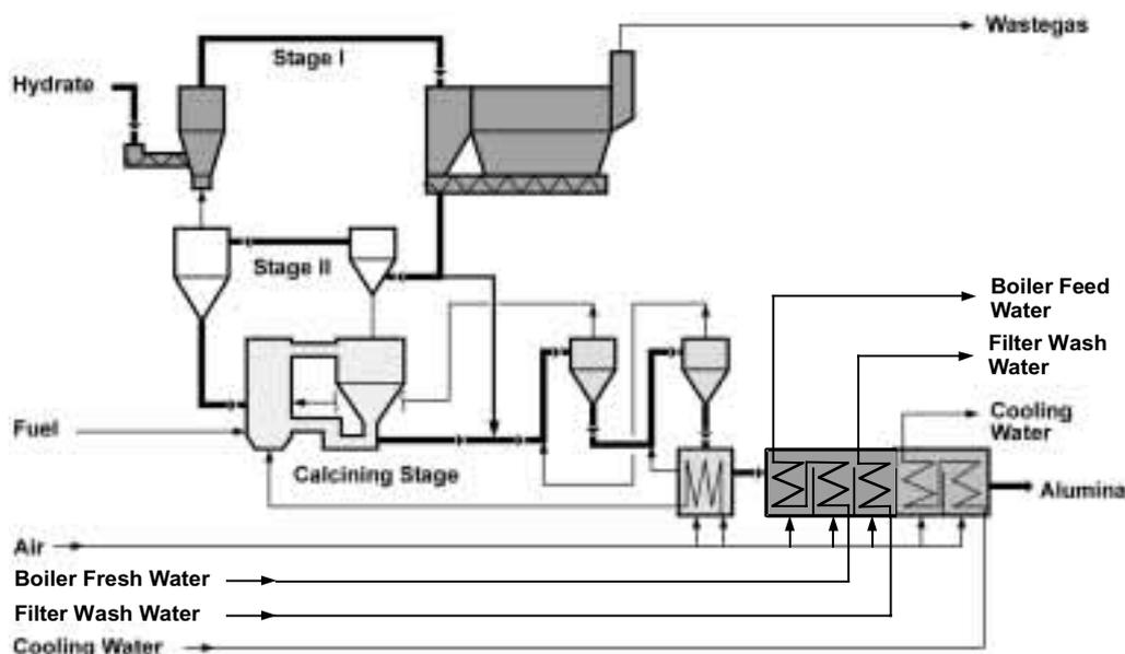
Figure 5 — Pre-heating of Filter Wash and Boiler Feed Water
