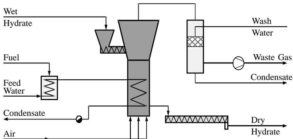
Figure 7 — Pilot Plant — Indirect Hydrate Dryer Flow Sheet, Capacity 1–2 t/h
