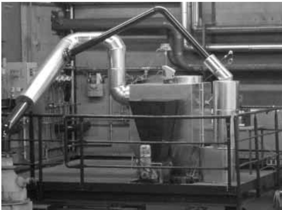
Figure 9 — Pilot Plant — Indirect Hydrate Dryer
