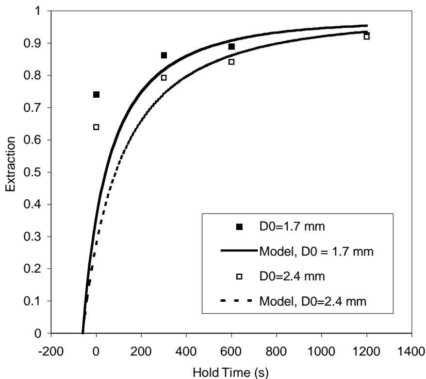
Figure 2 — Extraction versus Digestion Time
