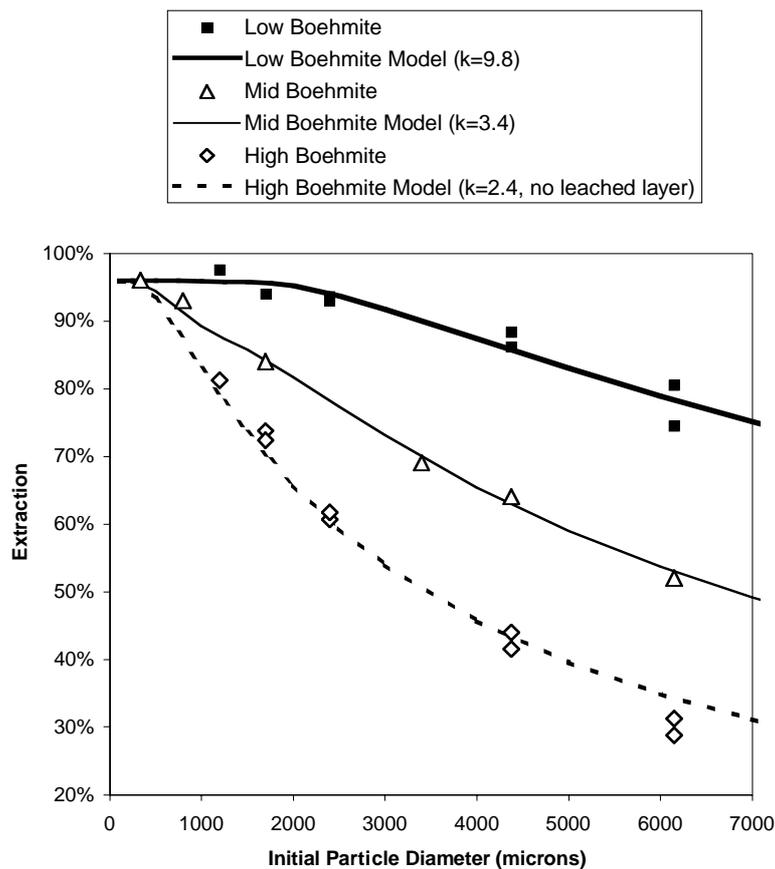
Figure 6 — Extraction versus Particle Size for Bauxites with Different Boehmite Contents
