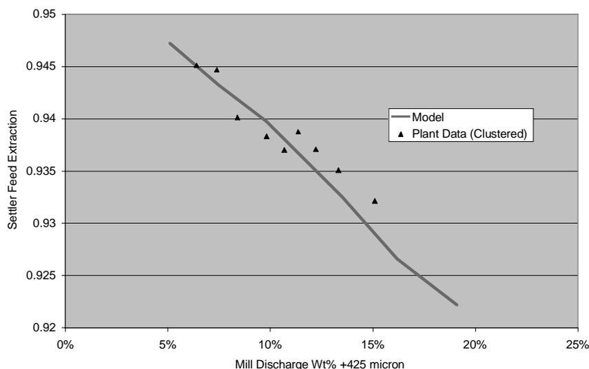
Figure 7 — Plant Digestion Extraction versus Grind
