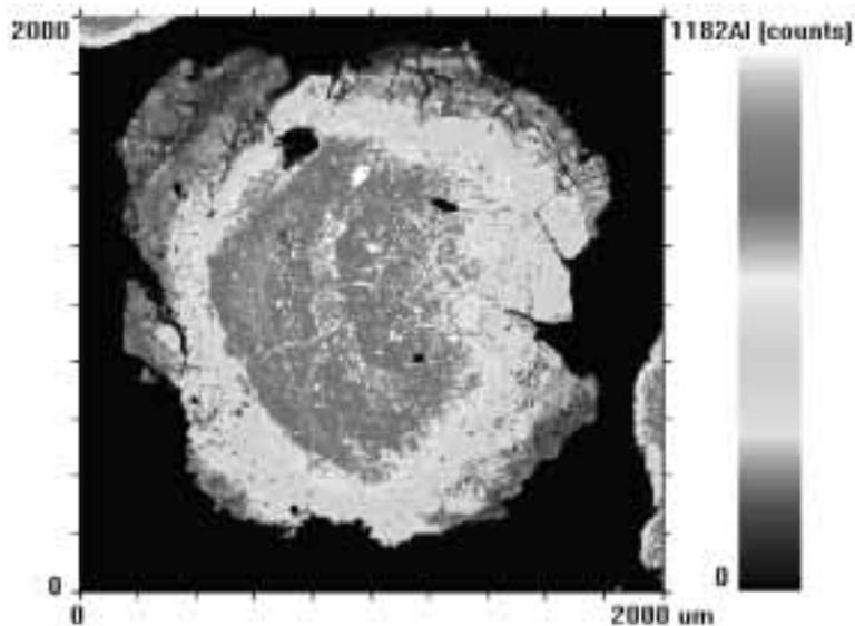
Figure 3 — Elemental SEM of Sectioned Bauxite Particle After Bomb Digestion
