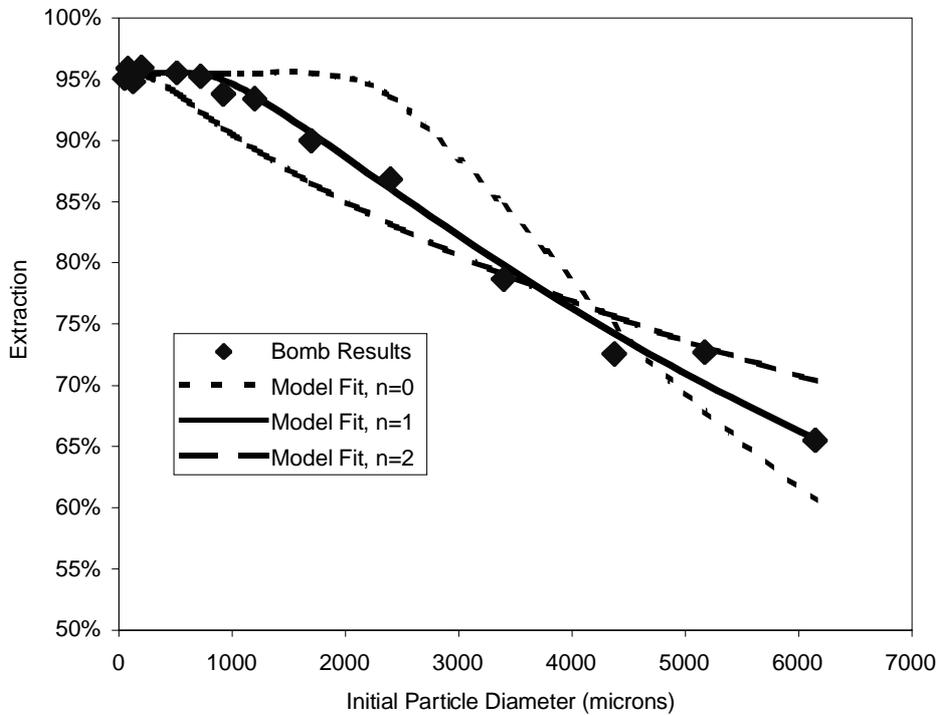
Figure 1 — Shrinking-Core Model Fit to Data in Table 1
