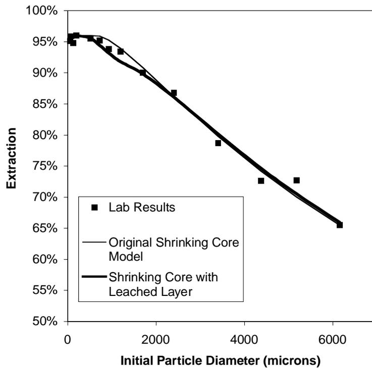
Figure 5 — Revised Shrinking-Core Fit to Data in Table 1
