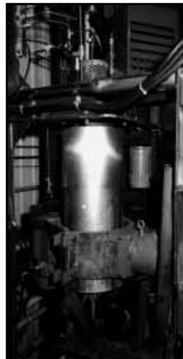
Figure 3 — Pilot Pressure Decanter
