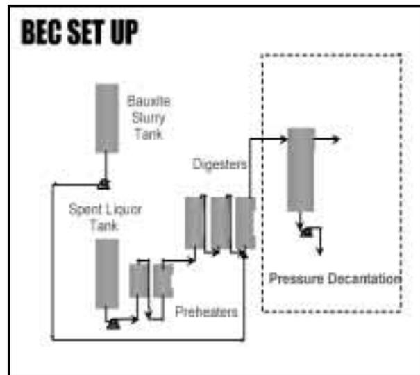
Figure 2 — Pressure decanter experimental set-up
