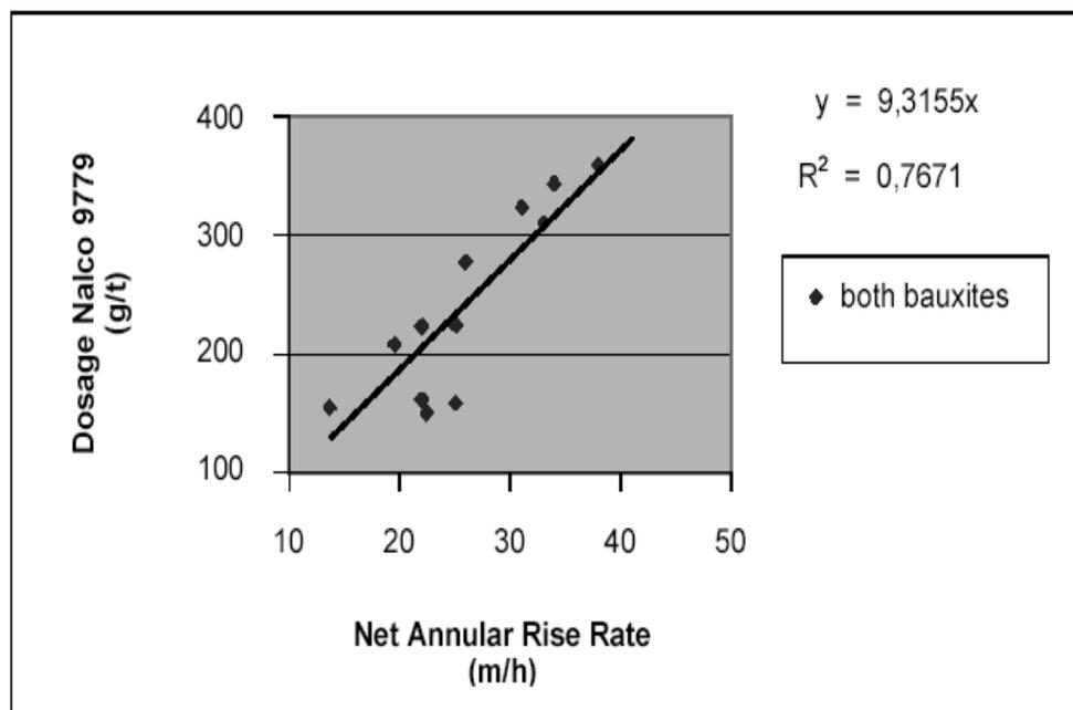
Figure 4 — Effect of Flocculent dosage on Net Rise Rate
