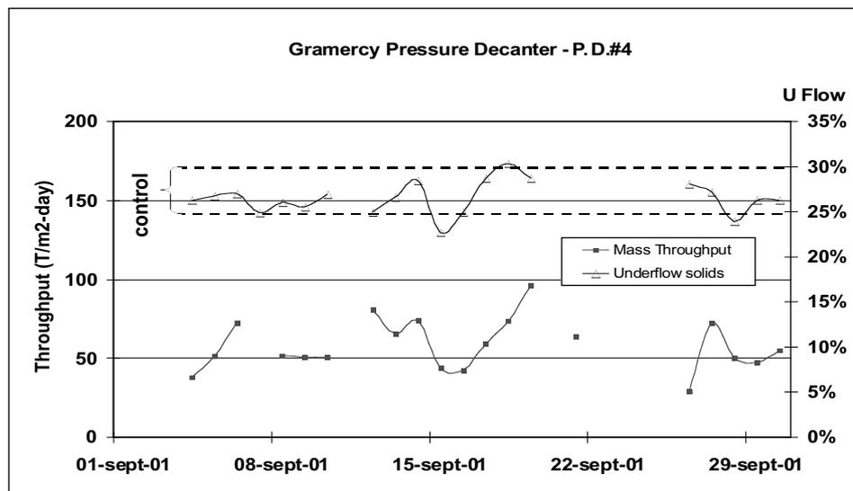
Figure 9 — P.D.#4 Operating Results — Throughput and Underflow — Sept. 2001
