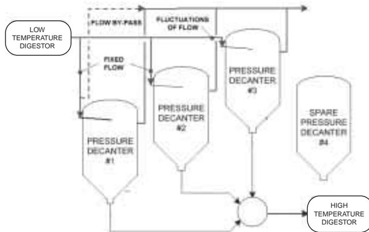
Figure 5 — Pressure decanters arrangement within Kaiser digestion circuit
