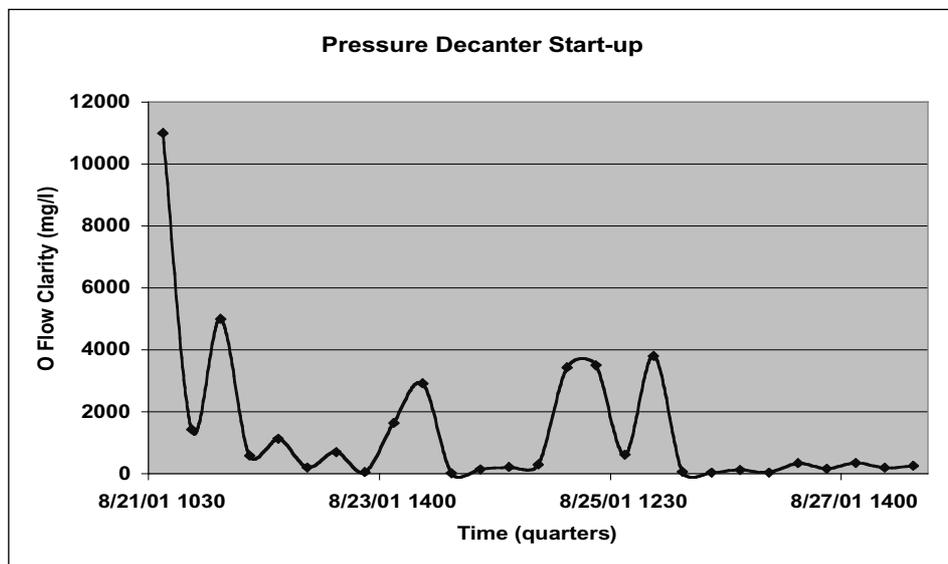
Figure 7 — O'Flow clarity on Start-up for Pressure Decanter #4
