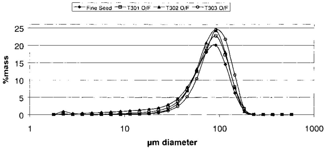
Figure 2 — PSD Evolution in Agglomerator Section-Actual Plant Data
