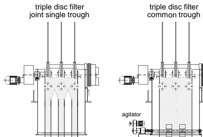
Figure 6 — Common trough design and "joint single trough" design
