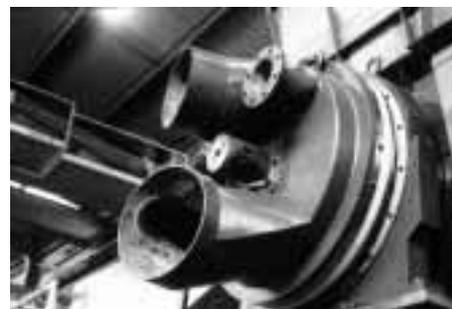
Figure 10 — High performance control head of the “Boozer” (L4-Type)
