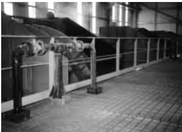
Figure 3 — Five triple-disc "Boozer" disc filters arranged in the filter building of an Alumina refinery
