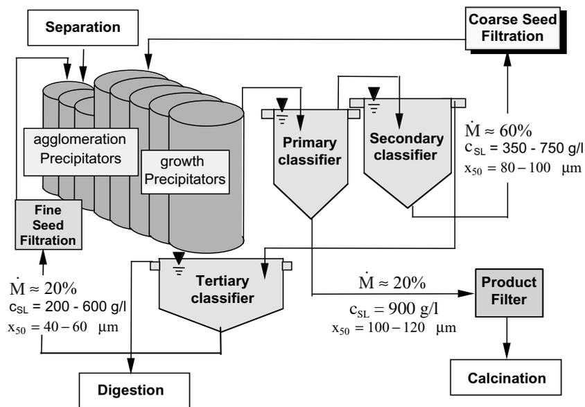
Figure 2 — Principle flow sheet of Al(OH)<sub>3</sub> precipitation and filtration in Alumina refineries
