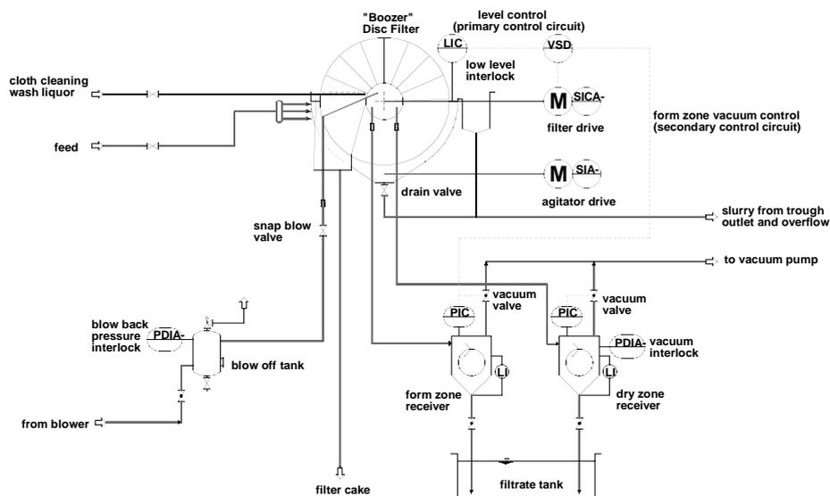
Figure 9 — Schematic P&I diagram of the High Performance Disc Filter “Boozer”
