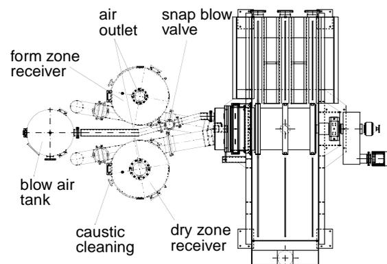
Figure 5 — Top view of a triple-disc “Boozer” filter with receivers, blow air tank and filtrate piping
