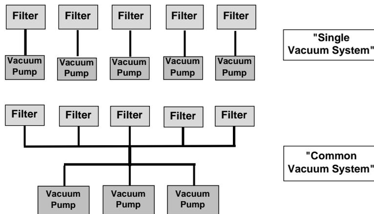
Figure 7 — Scheme of single and common vacuum system for a seed filter station
