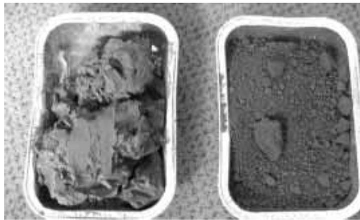
Figure 8 — Bauxite residue filter cakes: sticky and pasty with 35% moisture from vacuum filtration, dry and sand-like bulk material with 23% moisture from Hi-Bar® steam pressure filtration.
