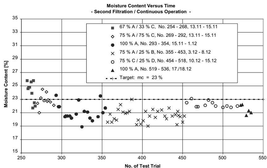
Figure 7 — Moisture content values of the “second-filtration” operation period for different bauxites.
