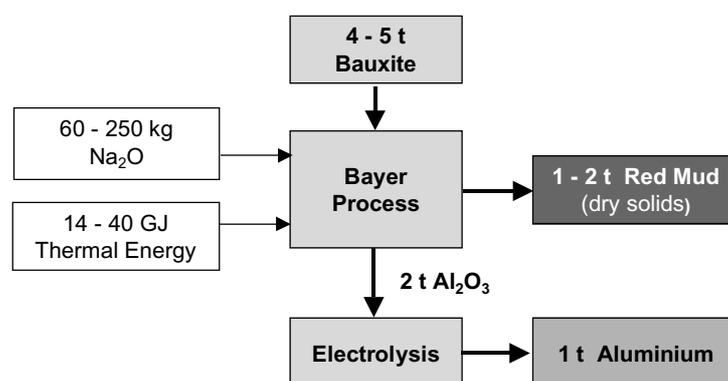
Figure 1 — Schematic flow sheet and material balance of aluminium production.
