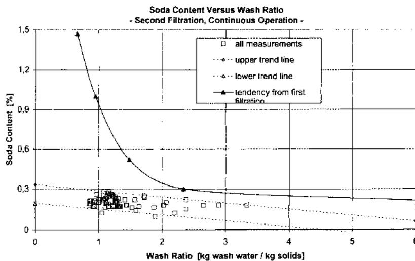
Figure 9 — Soda content versus wash ratio for “second-filtration” and “first-filtration”.
