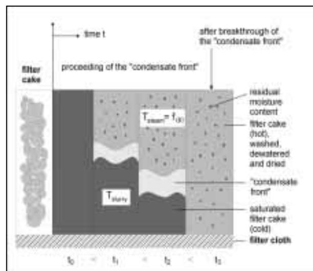
Figure 3 — Model of the “condensate front”.
