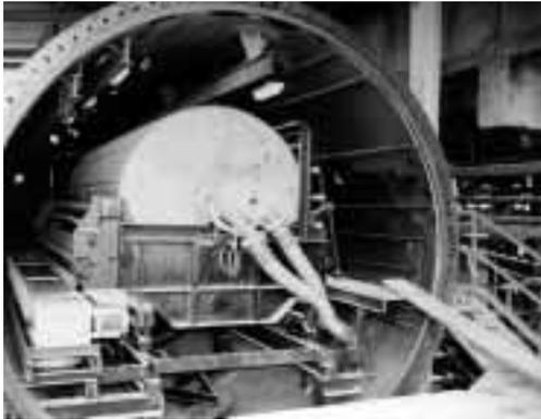
Figure 4 — Open pressure vessel of a Hi-Bar® Drum Filter Plant.
