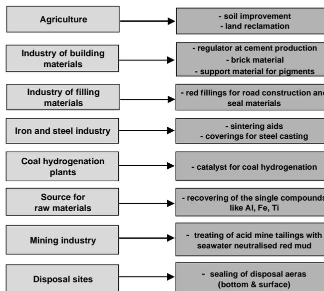
Figure 2 — Selection of some target industries and application possibilities for bauxite residue utilization.
