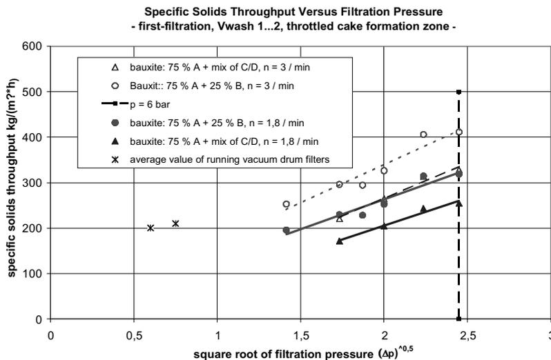
Figure 5 — Specific solids throughput as function of the square root of the pressure difference — “first-filtration” of 2 different bauxite types (filter speed n = 3 rpm and n = 1.8 rpm).
