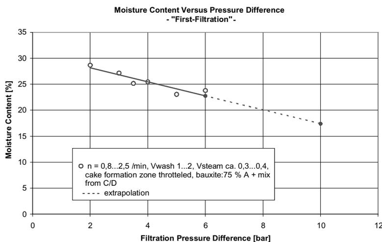
Figure 6 — Moisture content as a function of the filtration pressure difference.
