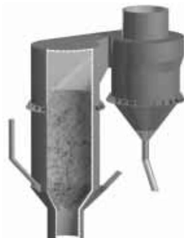
Figure 2B — Gas Suspension Calciner Furnace
