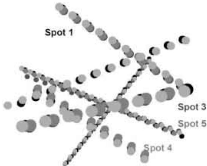
Figure 6 — Kikuchi patterns of radial gibbsite. Schematic of the overlaid Kikuchi patterns, from spots 1,3,4,5, is shown at the bottom (the use of dots is to aid comparison of the positions of the main diffraction lines in the Kikuchi patterns).
