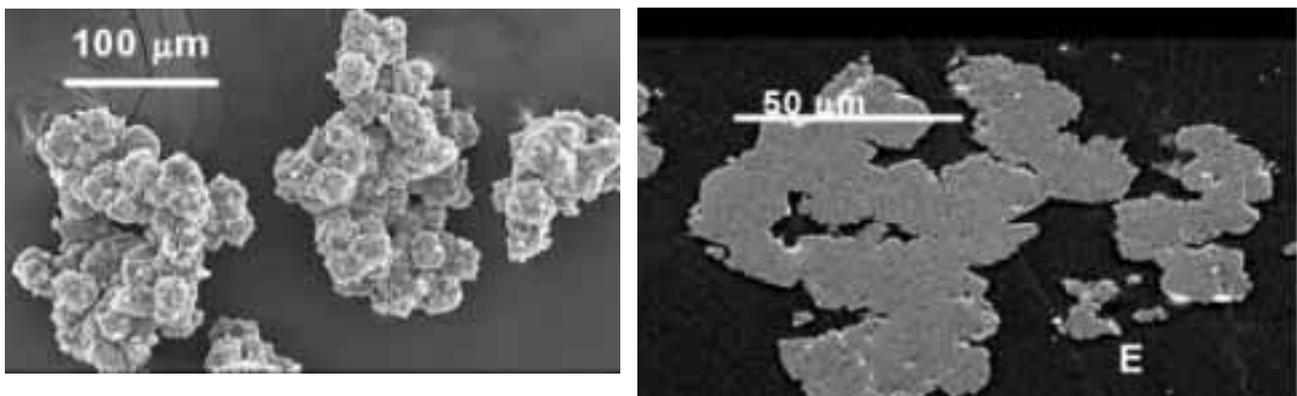
Figure 4 — SEM images of TC6D hydrate, grain-mount and sectioned and polished mount.
