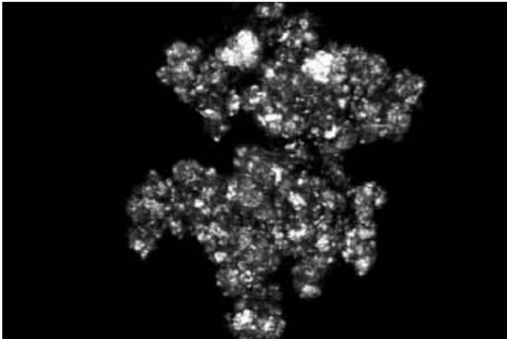
Figure 3 — Combined scanning laser confocal microscopy images of the sections from the TC6D hydrate (the software obtains an image by scanning through the "z" slices to obtain the maximum intensity value at each "x-y" pixel and then combining these to form a picture).
