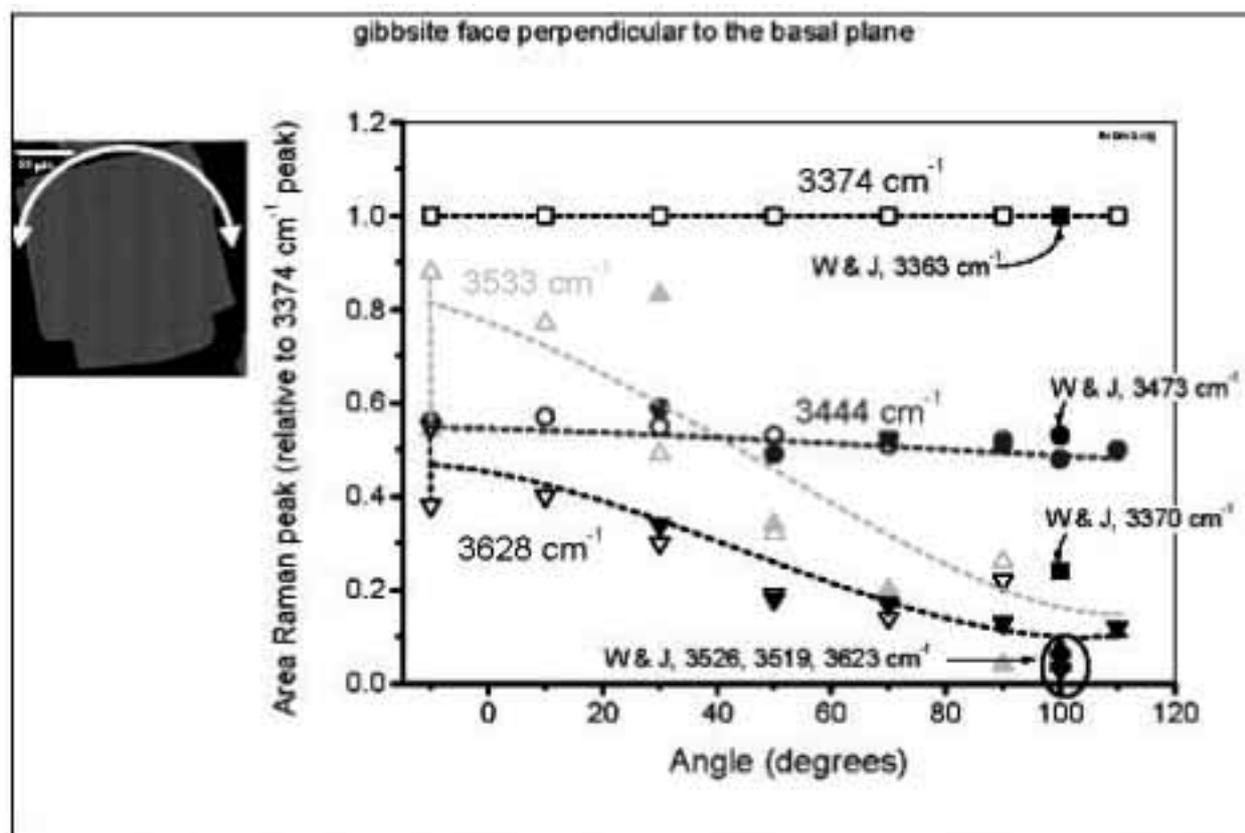
Figure 7 — Effect of crystal orientation: rotating the gibbsite crystal by a known angle about the axis shown. The data by Wang and Johnson (2000), for the  $a(bc)a$  orientation, is included for comparison (a description of the terminology used by Wang and Johnson can be found in their paper).
