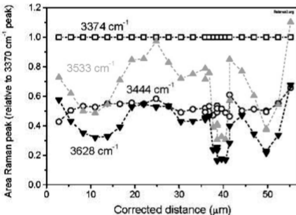
Figure 9 — Relative hydroxyl peak areas in the Raman spectra of gibbsite along the line shown in Figure 8a, b.
