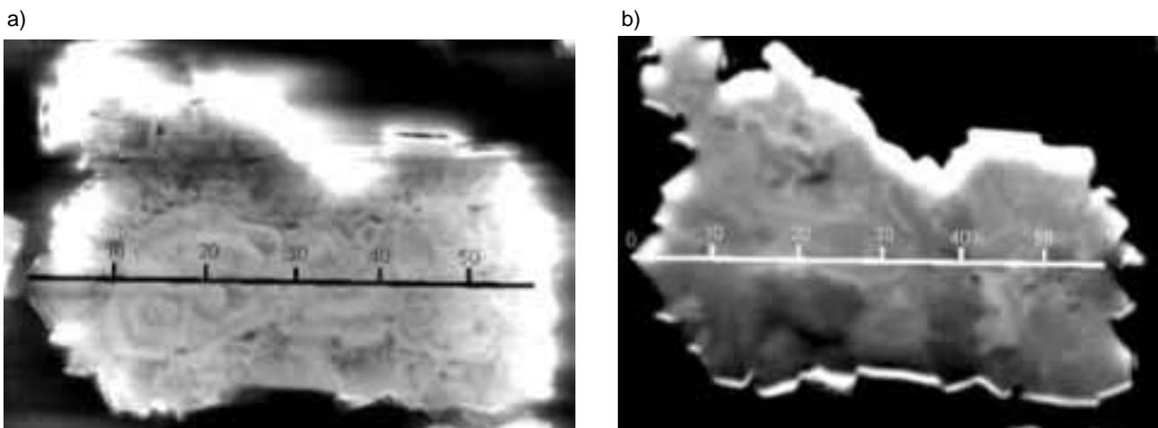
Figure 8 — Electron microscope images of CC12T7 hydrate agglomerate a) charge contrast image of sectioned and polished sample and b) orientation contrast image of the same grain examined in a).
