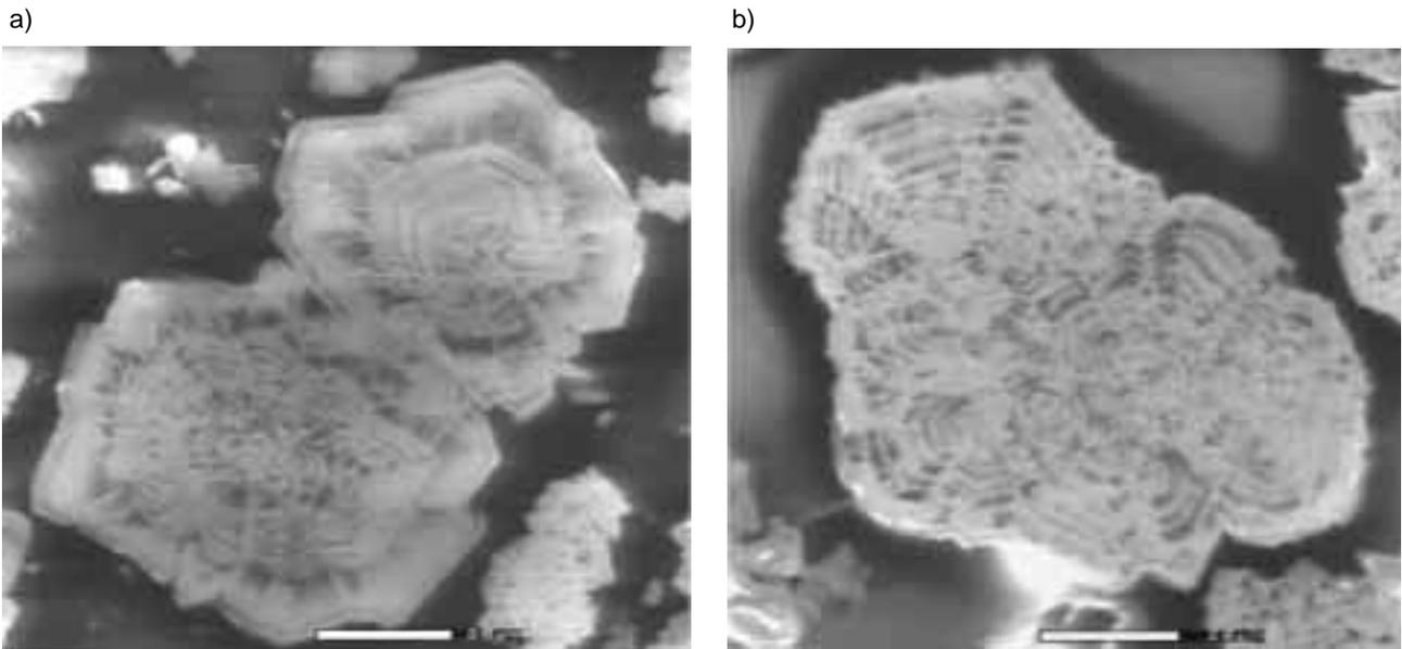
Figure 5 — Charge contrast images of a) Alcoa C-31 hydrate b) laboratory-prepared hydrate (B3-50).
